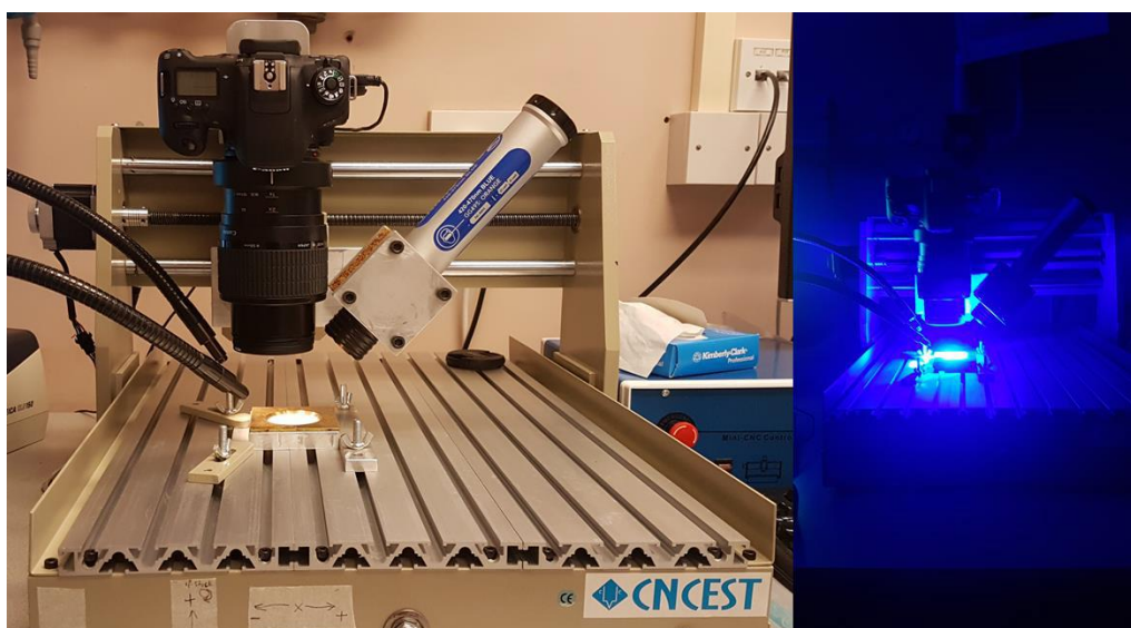
Figure S5. Experimental set-up of the digital imaging acquisition system using white light and blue light (420-470 nm).
