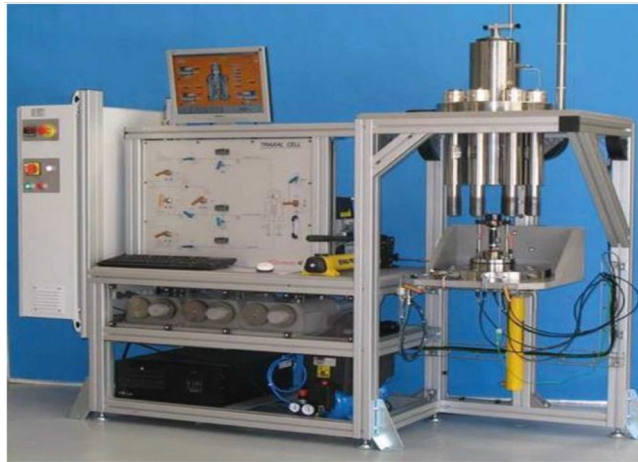
Supplementary Figure S3 The servo-controlled rheology testing machine
