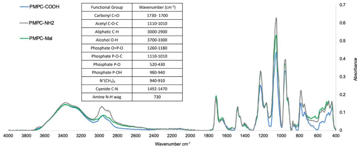
**Supplemental Figure 1. FT-IR spectra of PMPC-COOH, deprotected PMPC, and PMPC-Mal.**
