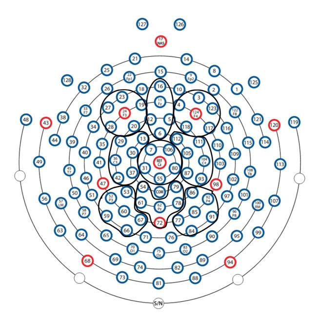
Channel layout of the Hydrocel Geodesic Sensor Net (128 channels). Channels selected for each of the 9 regions of interest have been circled.
