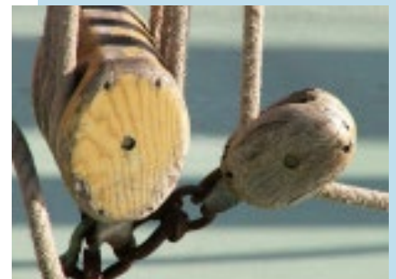
Pulleys used to lift loads on a ship. Credit: Wikimedia Commons
