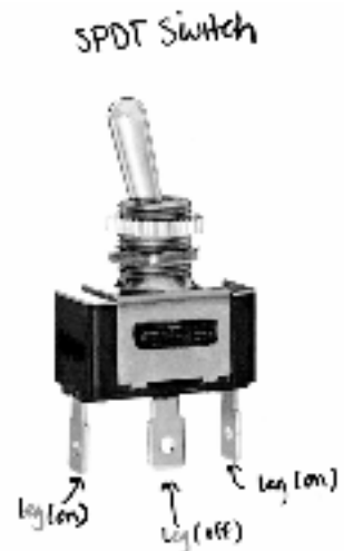
SPDT switch. Note the legs to which you will attach wires.
