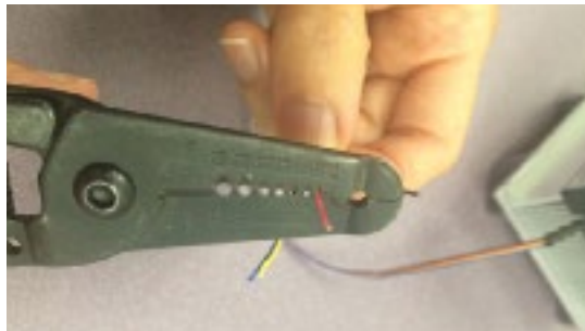
Wire strippers should snugly enclose the wire without nicking the wire.
