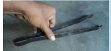
Tongs are an example of a lever . Credit: Wikimedia Commons
