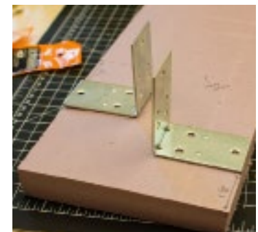
Make sure to stagger the L-brackets. Credit: Eurah Ko
