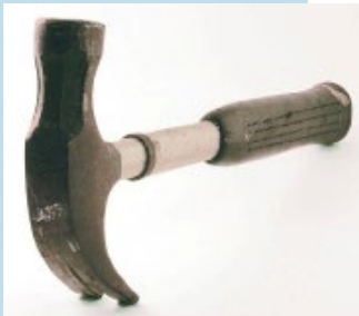
Hammers help you do work by making your swing longer and amplifying force .
