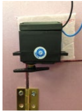
Make sure the motor arms are facing down. Credit: WGBH
