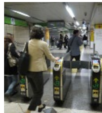
A swipe card triggers a switch to rotate these train station turnstiles and lock them after one turn. Credit: Wikimedia Commons
