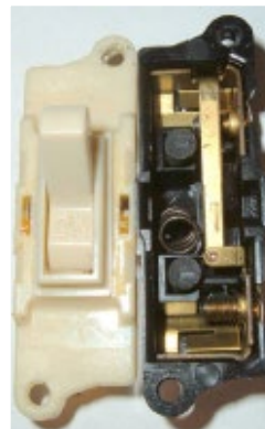
Inside a light switch. Credit: Wikimedia Commons
