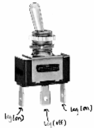
SPDT switch. Note the legs to which you will attach wires.
