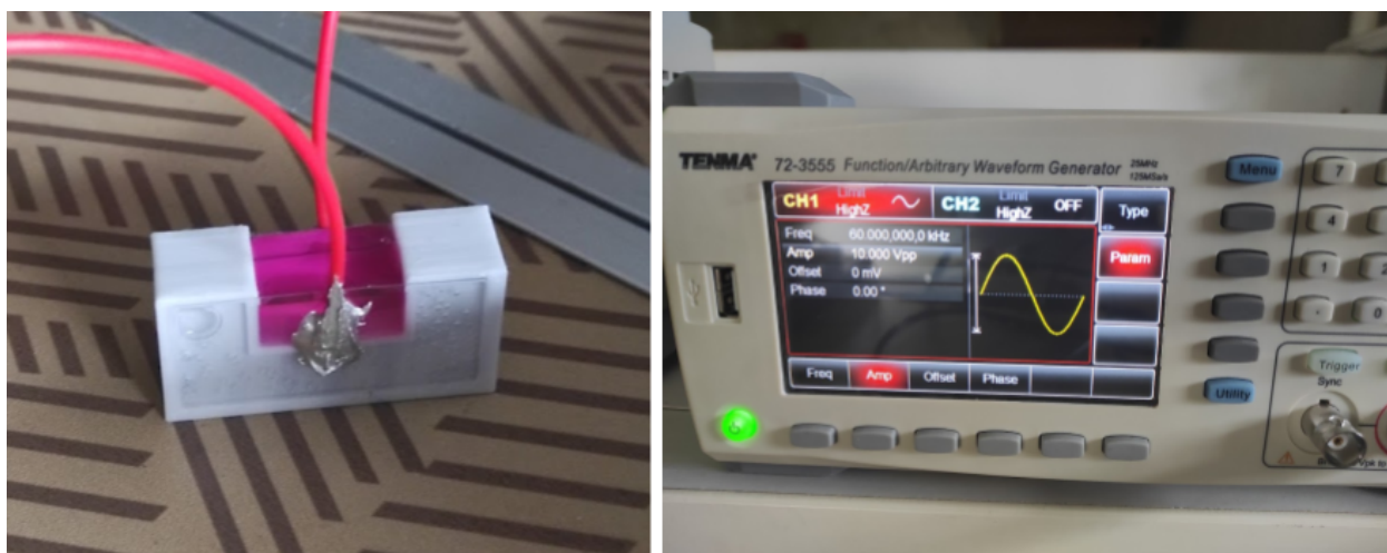
Figure S11 - Left: C-Coupled electrical stimulation system test apparatus with two ITO PET electrodes as described. Right: Applied waveform and signal source.
