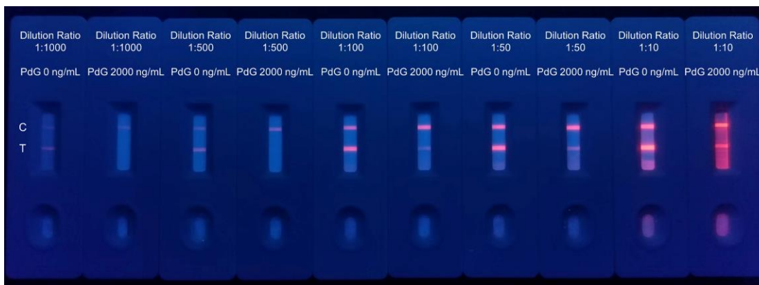
Figure S3 The detection image of TRFM-LFIA strip under ultraviolet irradiation in different TRFM-mAb dilution ratios.
