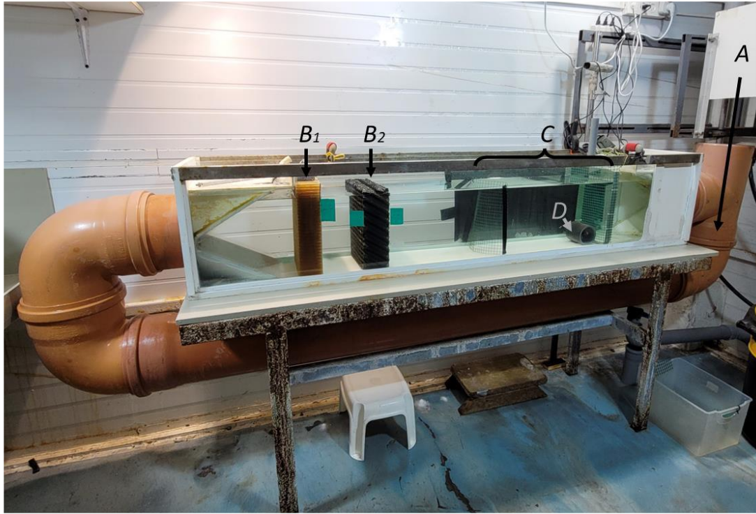
Figure S1: The recirculating flume: a motor A with a propeller thrusts seawater through the return pipe (orange) to the experimental arena C through two flow straighteners, B1 and B2. Flow speed is set using a calibrated controller (not shown) of the motor. Note the presence of the small pipe D, used as a shelter during trials with P. squamipinnis and Neopomacentrus miryae , replaced with a small coral skeleton for Dascyllus marginatus . (Photo credit: Hadar Ella.)
