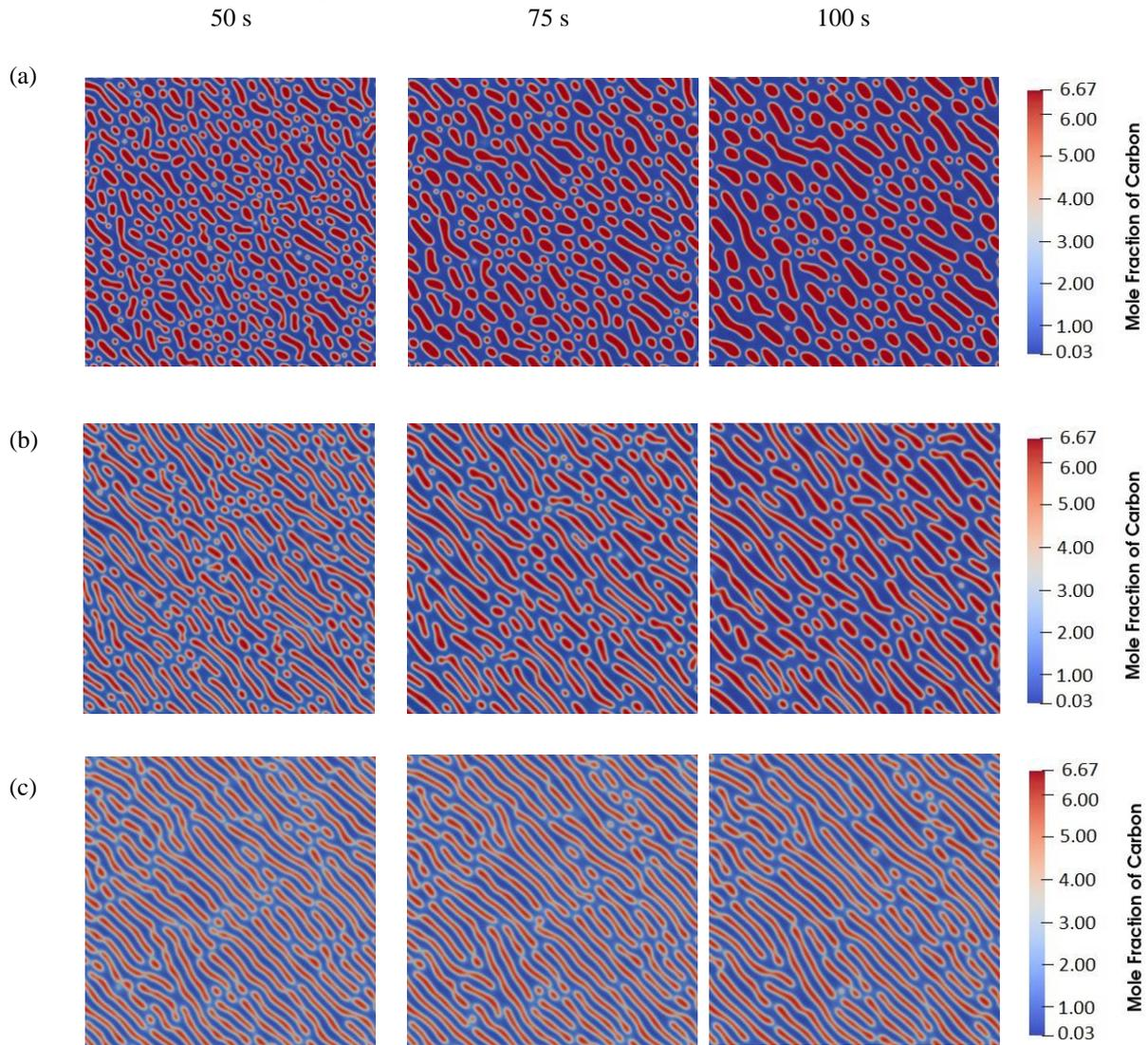
**Figure A 2 Phase evolution using a double-well potential with (a)  $A = 0.5$ , (b)  $A = 0.8$ , and (c)  $A = 1.8$  for 50 s, 75 s, and 100 s. The figure is colored by the concentration of red layers are cementite and blue matrix is ferrite.**
