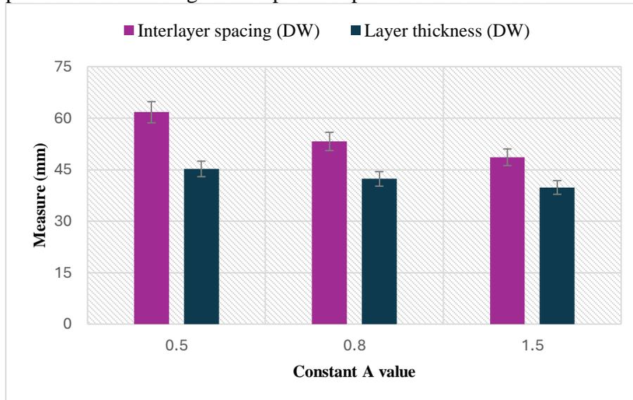
**Figure A 3 Interlamellar spacing, and layer thickness obtained from computation using double-well potential.**
