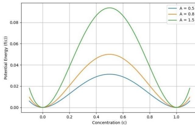
**Figure A 1** Change in potential relative to chemical composition at different values of  $A$ .
