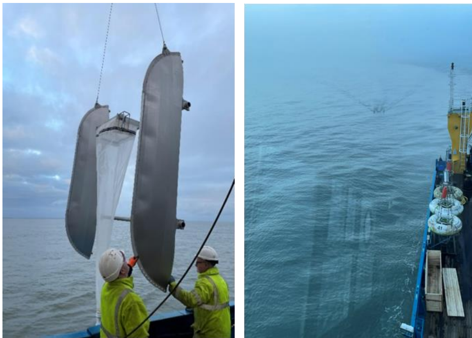
Figure S1: Neuston Catamaran with hulls and sampling net. Catamaran was towed on a 50 m cable behind the boat (starboard side) to avoid contamination and waves from the boat.
