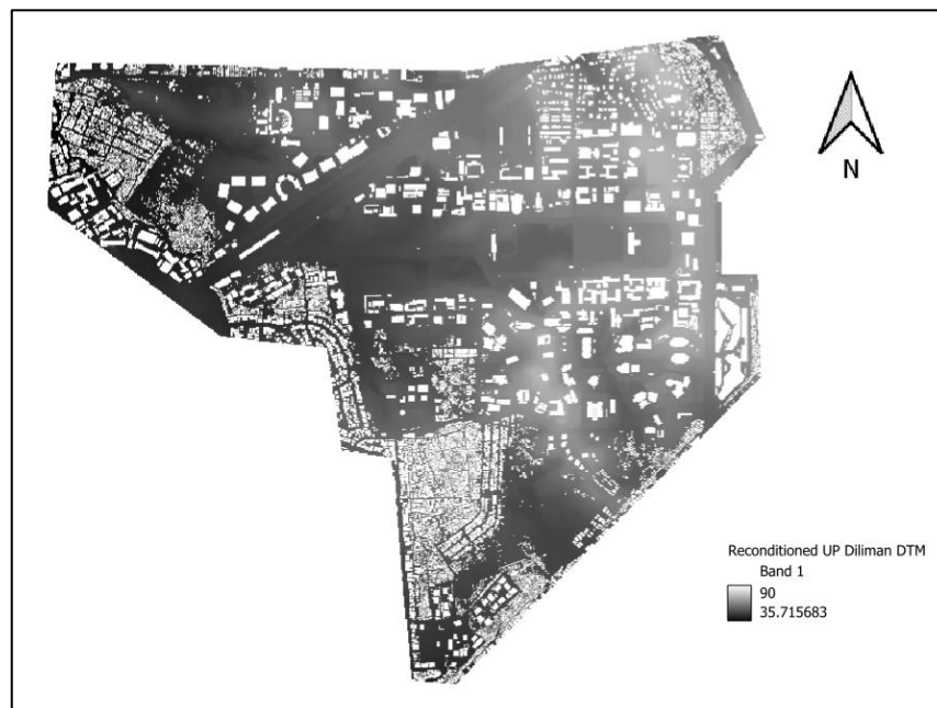
Supplementary Figure 2. Reconditioned DTM of UP Diliman.
