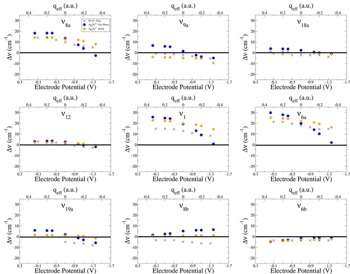
Supplementary Figure S15 Experimental wavenumber shifts  $\Delta\nu$  (crosses) and PW91/LanL2DZ/6-311G(d,p) calculated values  $\Delta\nu$  from isolated (blue) and solvated (PCM, orange)  $[\text{Ag}_n\text{Py}]^q$  complexes.
