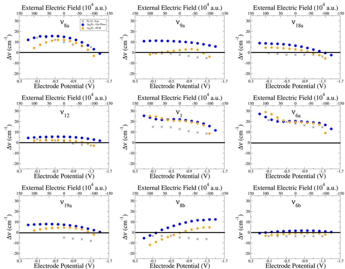
Supplementary Figure S25 Experimental wavenumber shifts  $\Delta\nu$  (crosses) and M06-HF/LanL2DZ calculated values under an external electric field from isolated (blue) and solvated (PCM, orange) [Ag<sub>2</sub>Py]<sup>0</sup> complex.
