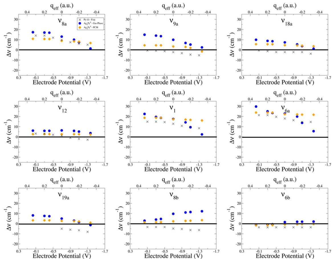
Supplementary Figure S16 Experimental wavenumber shifts  $\Delta\nu$  (crosses) and M06-HF/LanL2DZ/6-311G(d,p) calculated values  $\Delta\nu$  from isolated (blue) and solvated (PCM, orange)  $[\text{Ag}_n\text{Py}]^q$  complexes.
