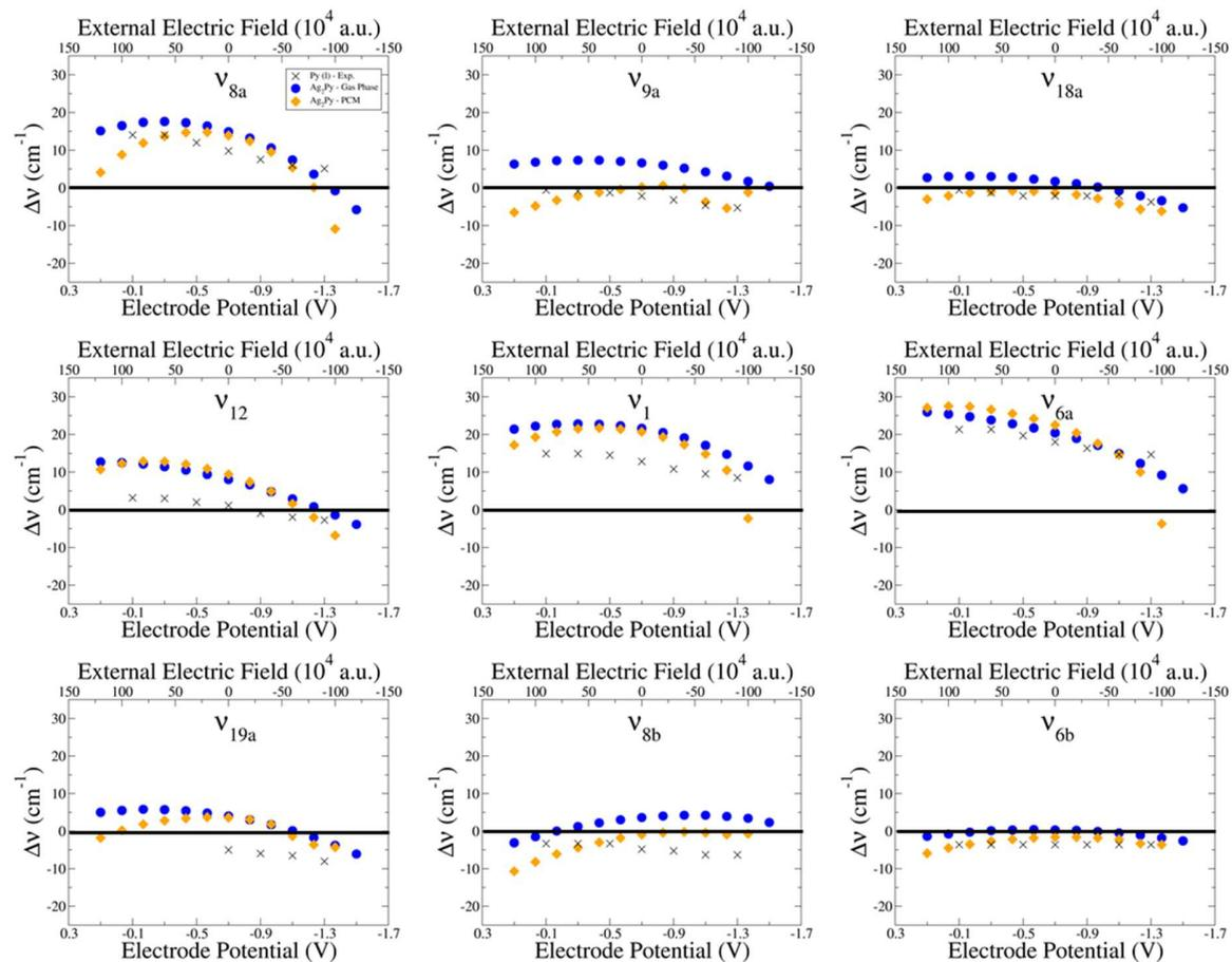
Supplementary Figure S23 Experimental wavenumber shifts  $\Delta\nu$  (crosses) and B3LYP/LanL2DZ calculated values under an external electric field from isolated (blue) and solvated (PCM, orange) [Ag<sub>2</sub>Py]<sup>0</sup> complex.
