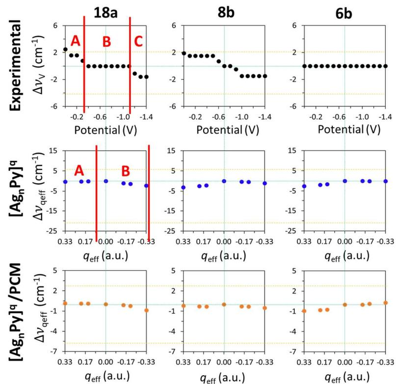
Supplementary Figure S7 Tuning of the experimental wavenumbers of pyridine vibrations by the electrode potential (top) and of the B3LYP/LanL2DZ calculated wavenumbers by the effective charge of isolated [Ag<sub>n</sub>Py]<sup>q</sup> complexes (middle) or in a PCM environment (bottom).
