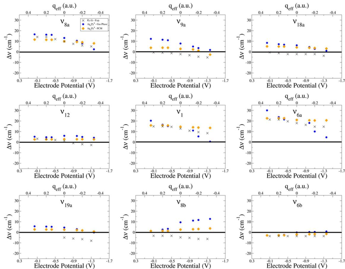
Supplementary Figure S13 Experimental wavenumber shifts  $\Delta\nu$  (crosses) and M06-HF/LanL2DZ/6-31G(d) calculated values  $\Delta\nu$  from isolated (blue) and solvated (PCM, orange) [Ag<sub>n</sub>Py]<sup>q</sup> complexes.
