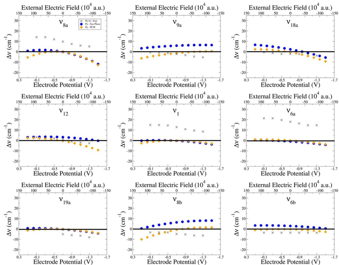
Supplementary Figure S19 Experimental wavenumber shifts  $\Delta\nu$  (crosses) and M06-HF/LanL2DZ calculated values under an external electric field from isolated (blue) and solvated (PCM, orange) pyridine.
