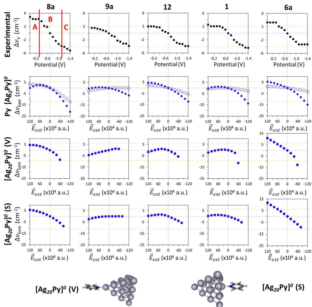
Supplementary Figure S6 Tuning of the experimental wavenumbers of pyridine vibrations on the electrode potential and of the B3LYP/LanL2DZ calculated wavenumbers on external electric fields of isolated Py (empty circles) and of  $[\text{Ag}_2\text{Py}]^0$ ,  $[\text{Ag}_{20}\text{Py}]^0$  (V) and  $[\text{Ag}_{20}\text{Py}]^0$  (S) complexes (full circles).
