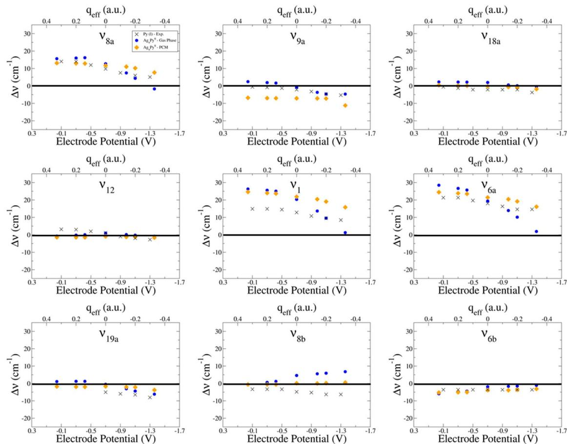
Supplementary Figure S12 Experimental wavenumber shifts  $\Delta\nu$  (crosses) and PW91/LanL2DZ/6-31G(d) calculated values  $\Delta\nu$  from isolated (blue) and solvated (PCM, orange)  $[Ag_nPy]^q$  complexes.
