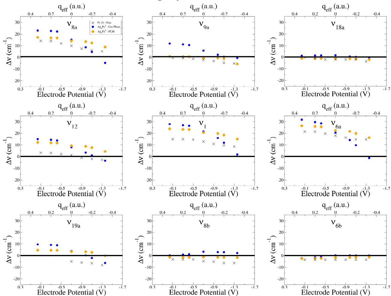
Supplementary Figure S8 Experimental wavenumber shifts  $\Delta\nu$  (crosses) and B3LYP/LanL2DZ calculated values  $\Delta\nu$  from isolated (blue) and solvated (PCM, orange)  $[\text{Ag}_n\text{Py}]^q$  complexes.
