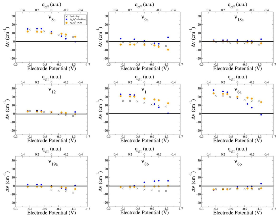
Supplementary Figure S11 Experimental wavenumber shifts  $\Delta\nu$  (crosses) and B3LYP/LanL2DZ/6-31G(d) calculated values  $\Delta\nu$  from isolated (blue) and solvated (PCM, orange) [Ag<sub>n</sub>Py]<sup>q</sup> complexes.
