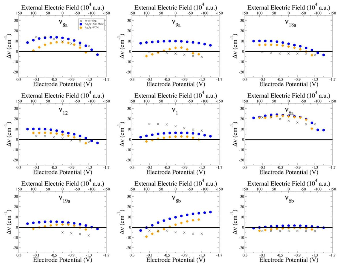
Supplementary Figure S28 Experimental wavenumber shifts  $\Delta\nu$  (crosses) and M06-HF/LanL2DZ/6-311G(d,p) calculated values under an external electric field from isolated (blue) and solvated (PCM, orange)  $[\text{Ag}_2\text{Py}]^0$  complex.
