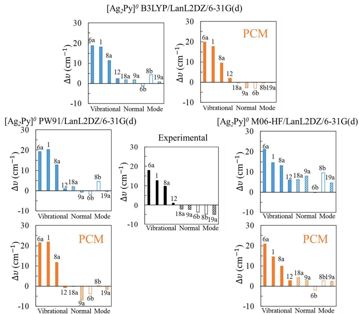
Supplementary Figure S3 Experimental (SERS at -0.7 V) wavenumber shifts  $\Delta\nu$  and calculated values at B3LYP, PW91 and M06-HF/LanL2DZ/6-31G(d) levels of theory from isolated and solvated (PCM)  $[\text{Ag}_2\text{Py}]^0$  complex.
