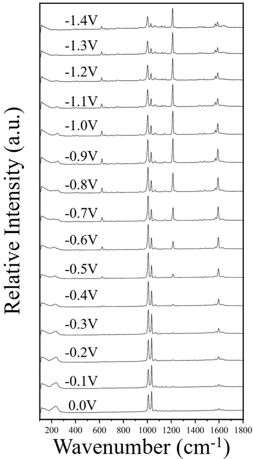
Supplementary Figure S1 Potential-dependent SERS spectra of Py aqueous solution (0.1 M) on silver electrode recorded in steps of 0.1 V. Excitation wavelength = 514 nm.
