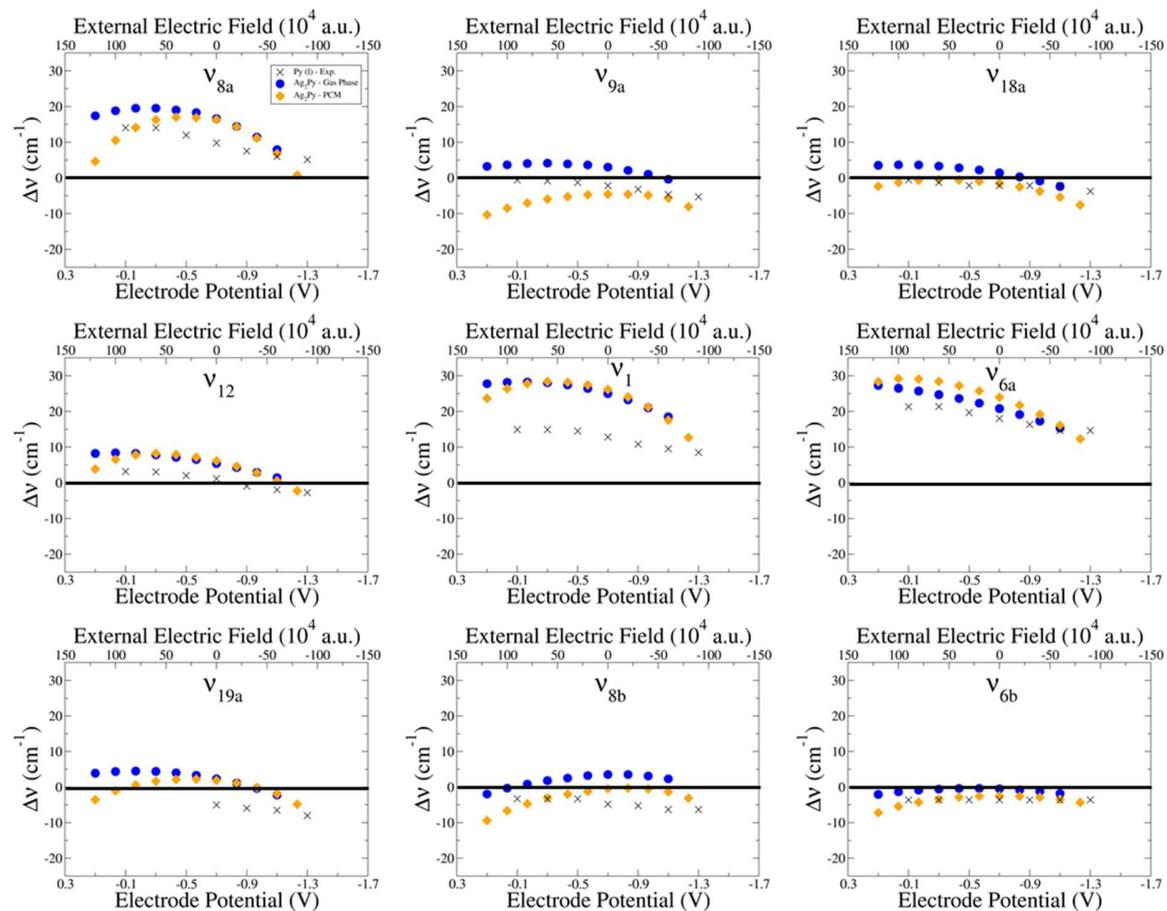
Supplementary Figure S24 Experimental wavenumber shifts  $\Delta\nu$  (crosses) and PW91/LanL2DZ calculated values under an external electric field from isolated (blue) and solvated (PCM, orange)  $[\text{Ag}_2\text{Py}]^0$  complex.
