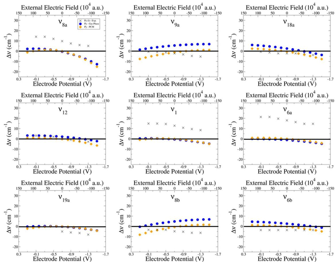
Supplementary Figure S21 Experimental wavenumber shifts  $\Delta\nu$  (crosses) and PW91/LanL2DZ/6-311G(d,p) calculated values under an external electric field from isolated (blue) and solvated (PCM, orange) pyridine.
