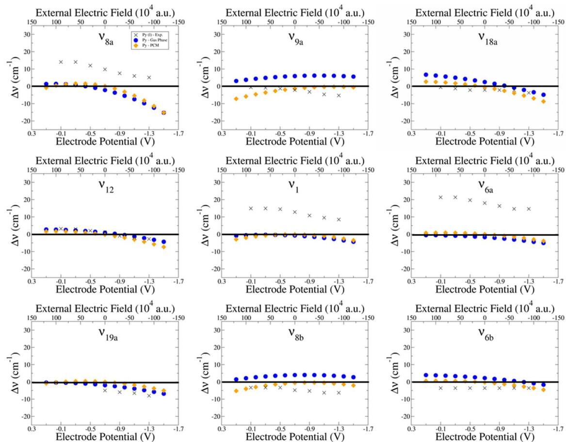
Supplementary Figure S18 Experimental wavenumber shifts  $\Delta\nu$  (crosses) and PW91/LanL2DZ calculated values under an external electric field from isolated (blue) and solvated (PCM, orange) pyridine.
