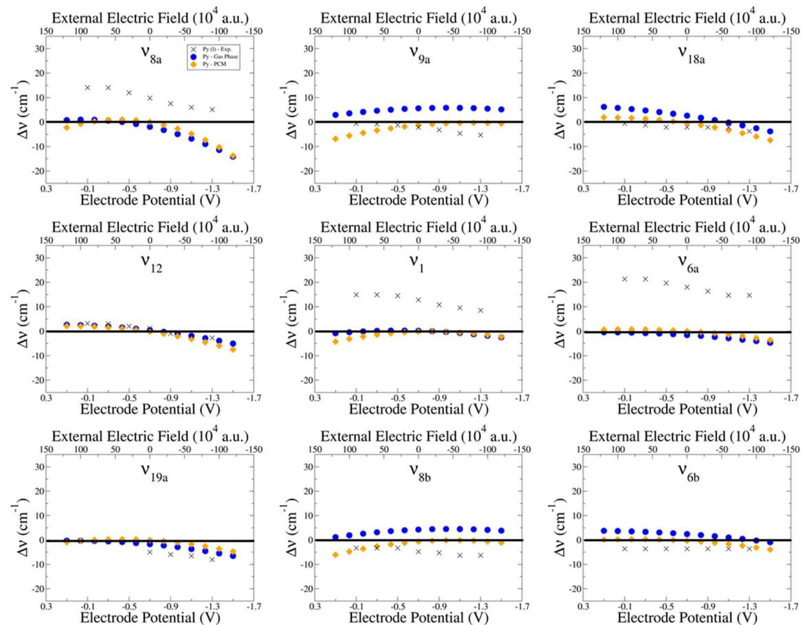
Supplementary Figure S17 Experimental wavenumber shifts  $\Delta\nu$  (crosses) and B3LYP/LanL2DZ calculated values under an external electric field from isolated (blue) and solvated (PCM, orange) pyridine.
