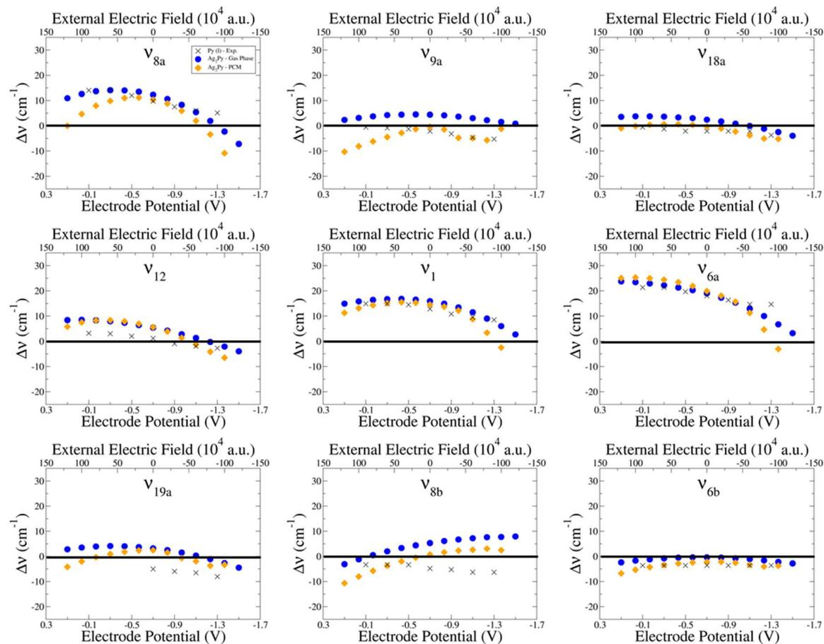
Supplementary Figure S26 Experimental wavenumber shifts  $\Delta\nu$  (crosses) and B3LYP/LanL2DZ/6-311G(d,p) calculated values under an external electric field from isolated (blue) and solvated (PCM, orange)  $[\text{Ag}_2\text{Py}]^0$  complex.
