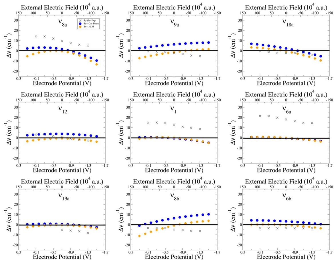
Supplementary Figure S22 Experimental wavenumber shifts  $\Delta\nu$  (crosses) and M06-HF/LanL2DZ/6-311G(d,p) calculated values under an external electric field from isolated (blue) and solvated (PCM, orange) pyridine.
