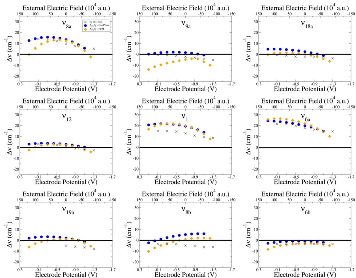
Supplementary Figure S27 Experimental wavenumber shifts  $\Delta\nu$  (crosses) and PW91/LanL2DZ/6-311G(d,p) calculated values under an external electric field from isolated (blue) and solvated (PCM, orange)  $[\text{Ag}_2\text{Py}]^0$  complex.
