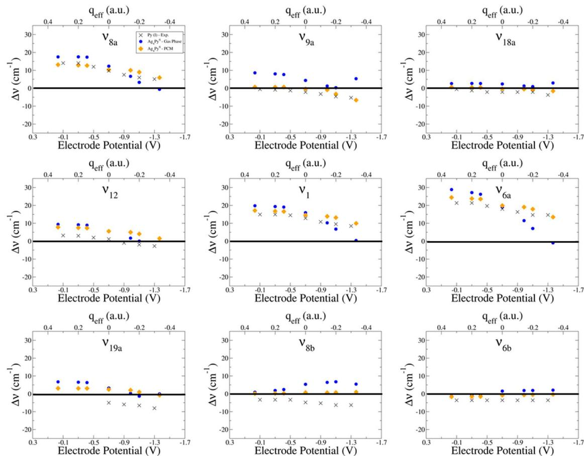
Supplementary Figure S14 Experimental wavenumber shifts  $\Delta\nu$  (crosses) and B3LYP/LanL2DZ/6-311G(d,p) calculated values  $\Delta\nu$  from isolated (blue) and solvated (PCM, orange)  $[\text{Ag}_n\text{Py}]^q$  complexes.
