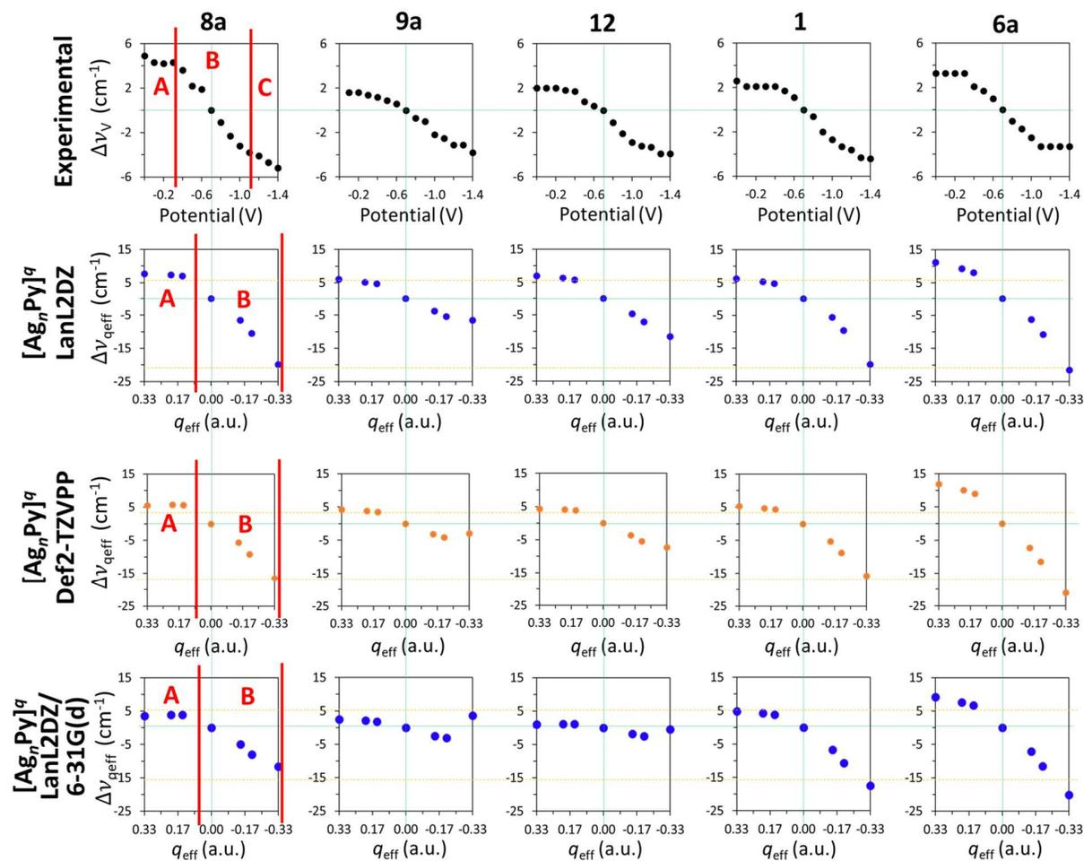
Supplementary Figure S5 Tuning of the experimental wavenumbers of pyridine vibrations by the electrode potential (top, black) and of the B3LYP/LanL2DZ (middle, blue), B3LYP/def2-TZVPP (middle, orange) or B3LYP/LanL2DZ/6-31G(d) (bottom, blue) calculated wavenumbers by the effective charge of isolated  $[Ag_nPy]^q$  complexes.
