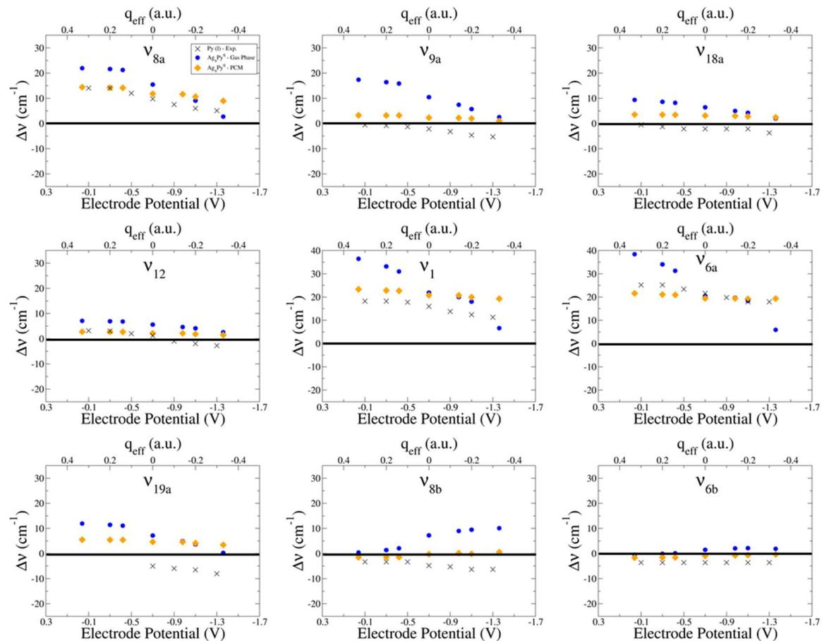
Supplementary Figure S10 Experimental wavenumber shifts  $\Delta\nu$  (crosses) and M06-HF/LanL2DZ calculated values  $\Delta\nu$  from isolated (blue) and solvated (PCM, orange)  $[Ag_nPy]^q$  complexes.
