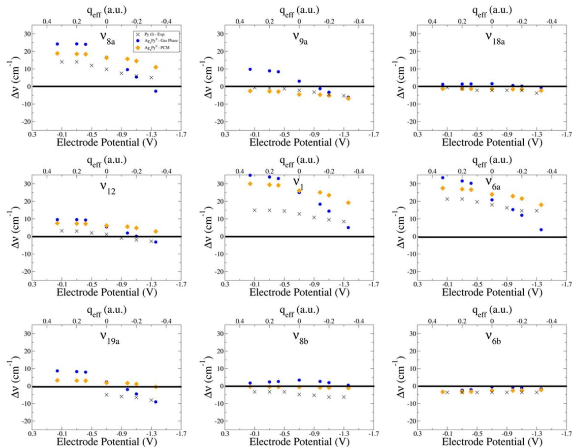
Supplementary Figure S9 Experimental wavenumber shifts  $\Delta\nu$  (crosses) and PW91/LanL2DZ calculated values  $\Delta\nu$  from isolated (blue) and solvated (PCM, orange) [Ag<sub>n</sub>Py]<sup>q</sup> complexes.
