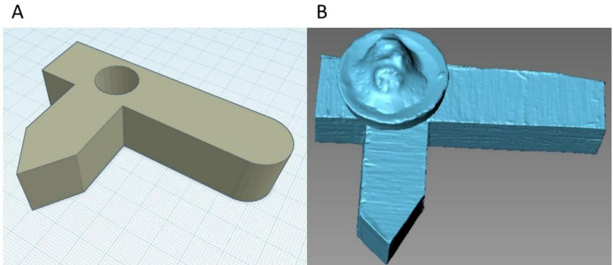
**Figure S2.** Custom-designed stand for coral fragments mounted on circular plugs. The stand has unique geometry on each side **(A)** for more effective scanning and a mounting spot **(B)** to securely hold the plug during scanning.
