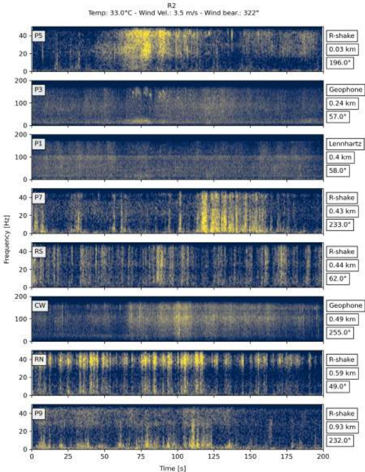
**Figure S4.** Spectrograms for seismic data as recorded during Reunion 2, plotted in order of distance of station from the event. Station names are labeled in top left of each panel. Details on the sensor, distance from reunion, and bearing from reunion location to station are labeled by the right side of each panel. Atmospheric temperature and wind conditions are stated at top of figure.
