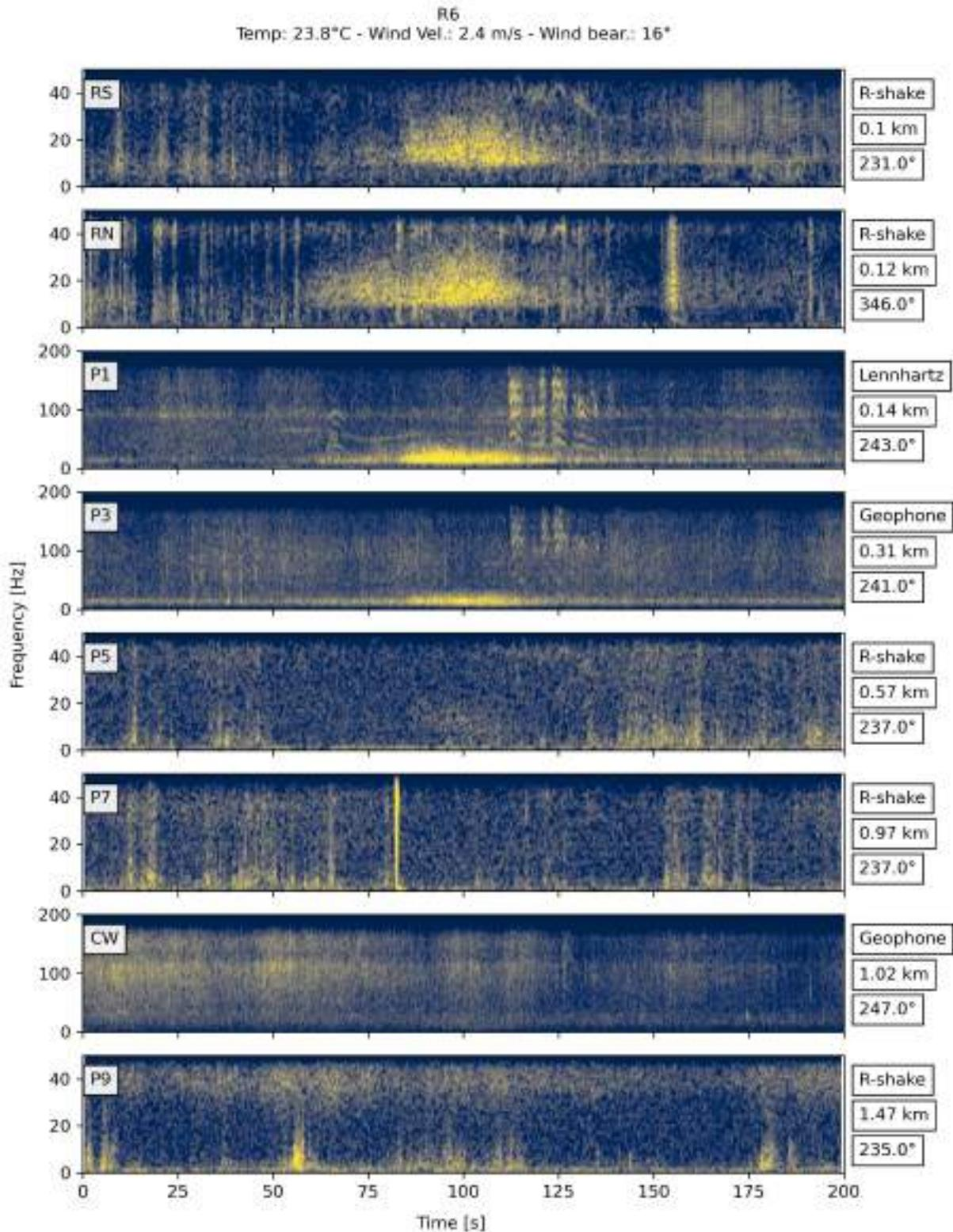
**Figure S12.** Spectrograms for seismic data as recorded during Reunion 6, plotted in order of distance of station from the event. Station names are labeled in top left of each panel. Details on the sensor, distance from reunion, and bearing from reunion location to station are labeled by the right side of each panel. Atmospheric temperature and wind conditions are stated at top of figure.
