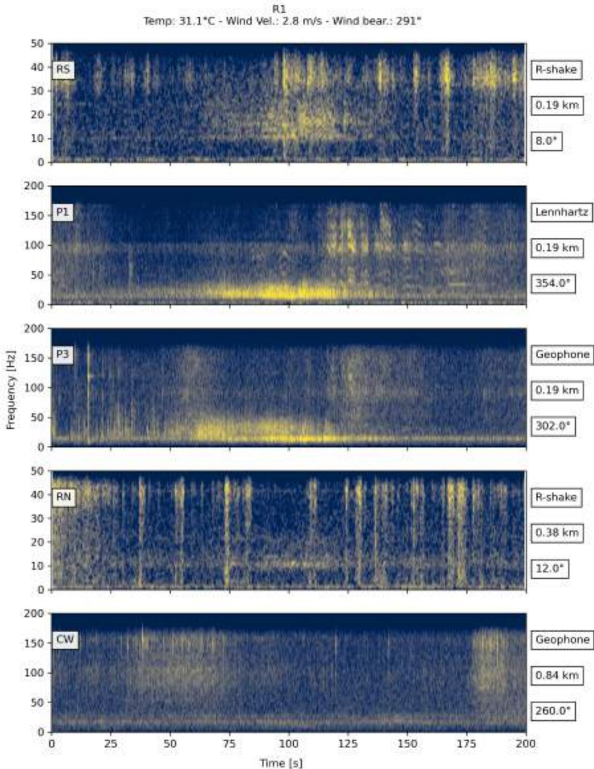
**Figure S2.** Spectrograms for seismic data as recorded during Reunion 1, plotted in order of distance of station from the event. Station names are labeled in top left of each panel. Details on the sensor, distance from reunion, and bearing from reunion location to station are labeled by the right side of each panel. Atmospheric temperature and wind conditions are stated at top of figure. Note that data from stations P5, P7, and P9 are not plotted here due to technical issues with the stations.
