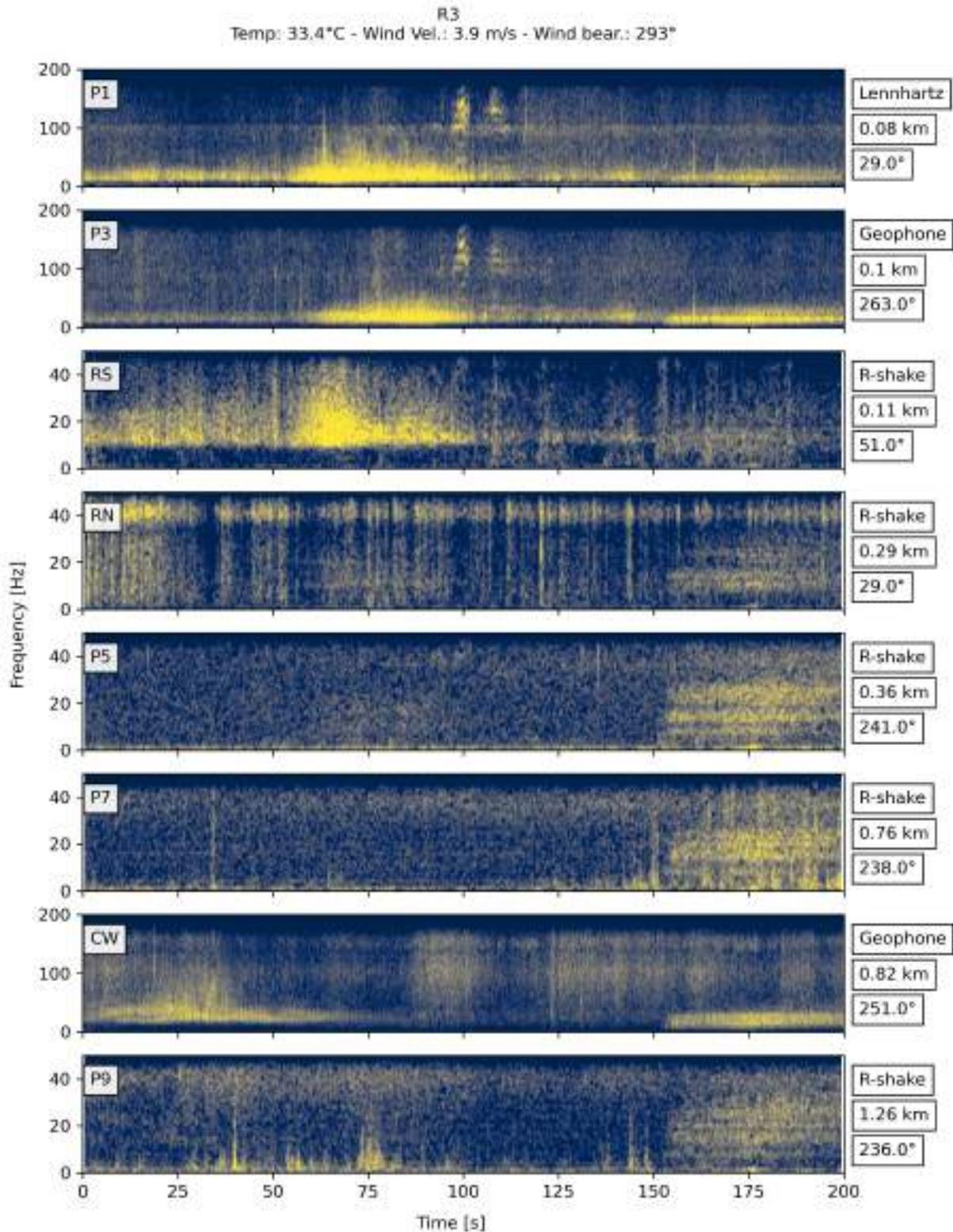
**Figure S6.** Spectrograms for seismic data as recorded during Reunion 3, plotted in order of distance of station from the event. Station names are labeled in top left of each panel. Details on the sensor, distance from reunion, and bearing from reunion location to station are labeled by the right side of each panel. Atmospheric temperature and wind conditions are stated at top of figure.
