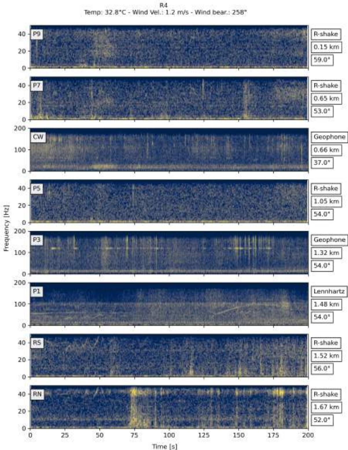
**Figure S8.** Spectrograms for seismic data as recorded during Reunion 4, plotted in order of distance of station from the event. Station names are labeled in top left of each panel. Details on the sensor, distance from reunion, and bearing from reunion location to station are labeled by the right side of each panel. Atmospheric temperature and wind conditions are stated at top of figure.
