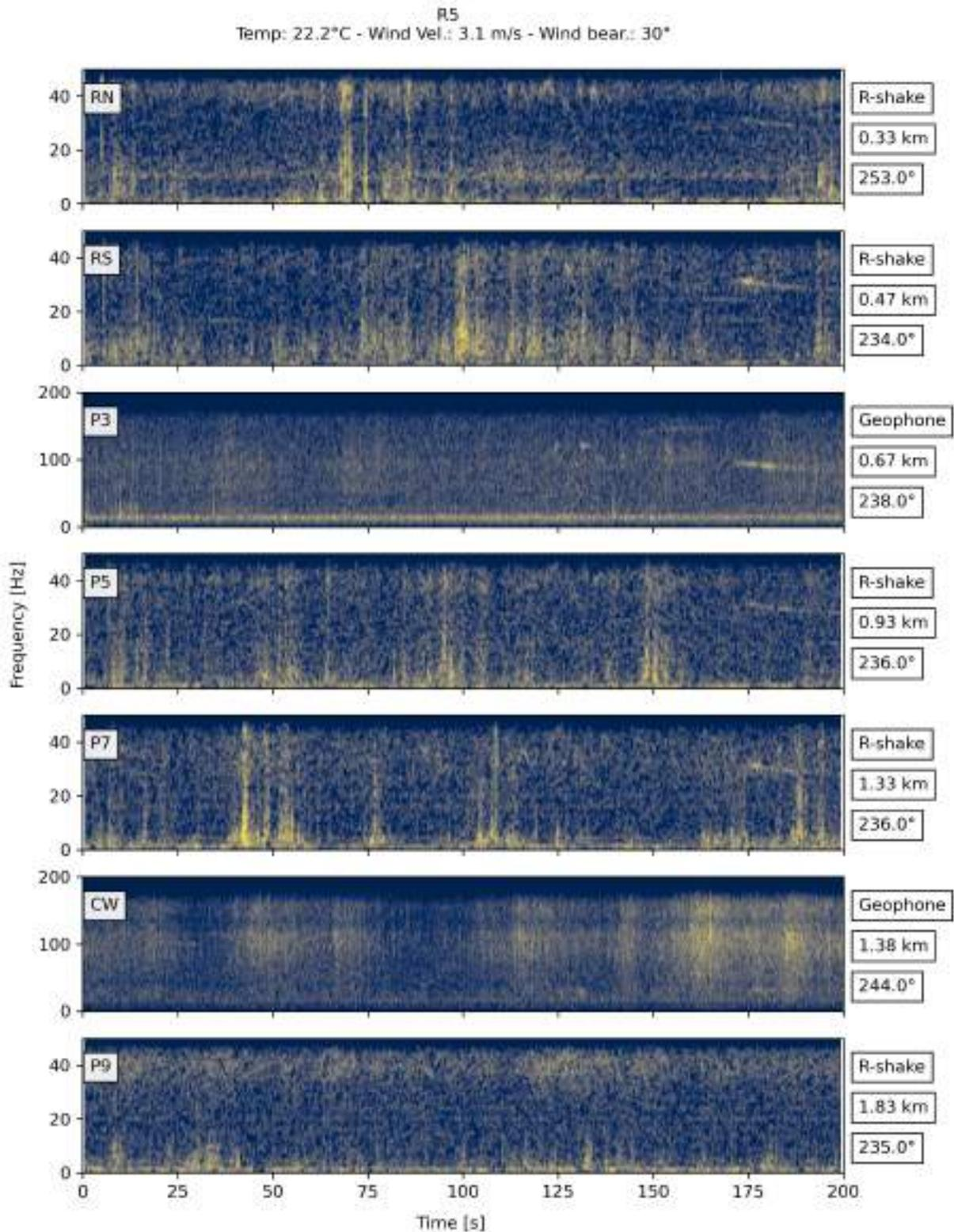
**Figure S10.** Spectrograms for seismic data as recorded during Reunion 5, plotted in order of distance of station from the event. Station names are labeled in top left of each panel. Details on the sensor, distance from reunion, and bearing from reunion location to station are labeled by the right side of each panel. Atmospheric temperature and wind conditions are stated at top of figure.
