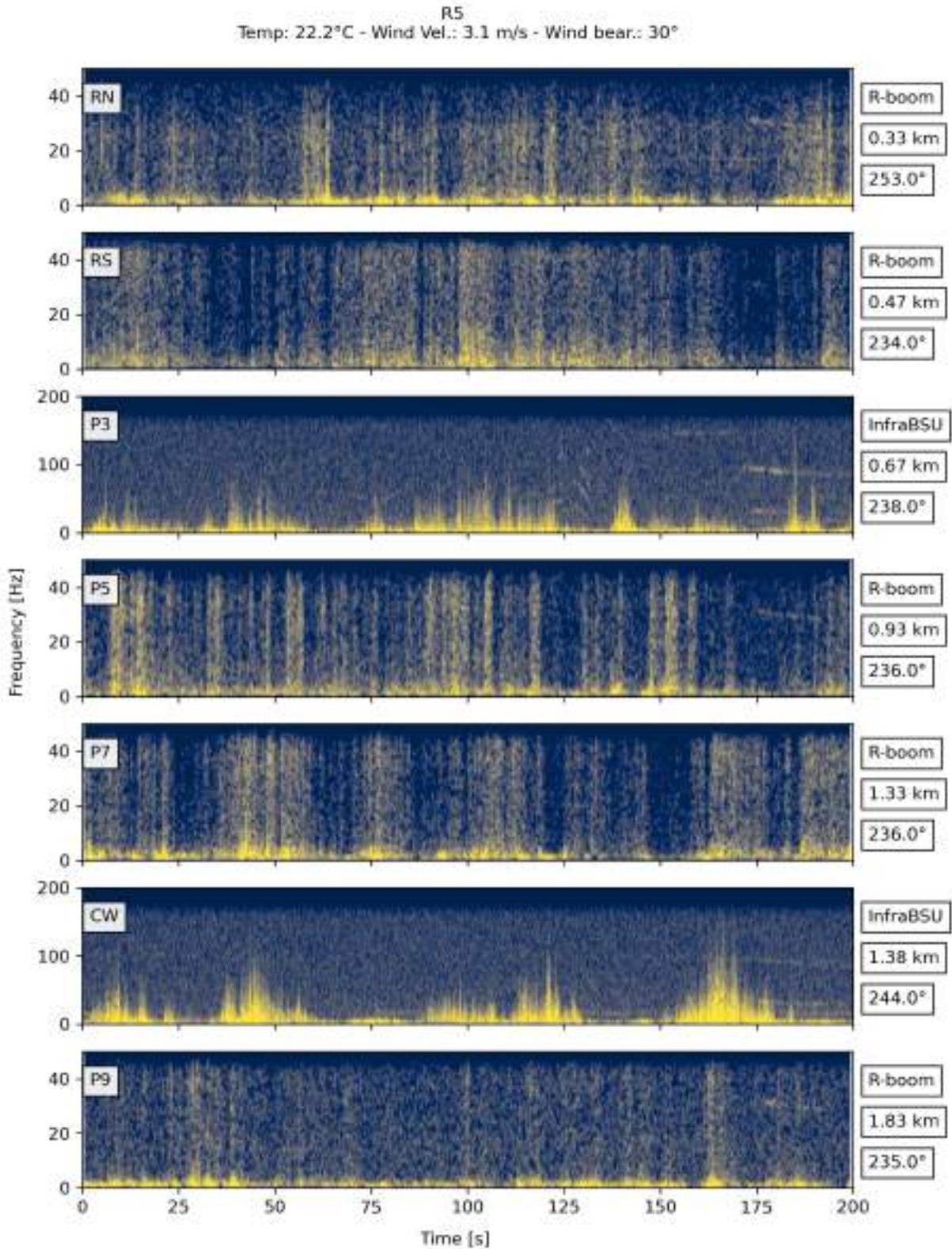
**Figure S11.** Spectrograms for acoustic data as recorded during Reunion 5, plotted in order of distance of station from the event. Station names are labeled in top left of each panel. Details on the sensor, distance from reunion, and bearing from reunion location to station are labeled by the right side of each panel. Atmospheric temperature and wind conditions are stated at top of figure. Note that station P1 is not plotted due to technical issues with the microphone.
