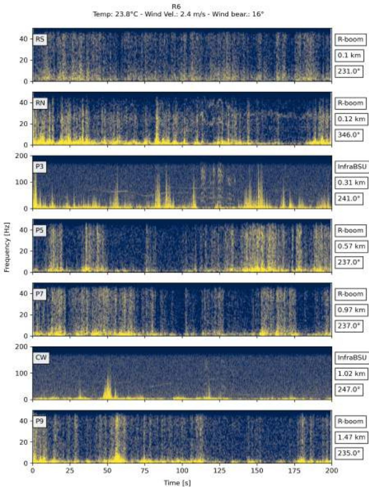
**Figure S13.** Spectrograms for acoustic data as recorded during Reunion 6, plotted in order of distance of station from the event. Station names are labeled in top left of each panel. Details on the sensor, distance from reunion, and bearing from reunion location to station are labeled by the right side of each panel. Atmospheric temperature and wind conditions are stated at top of figure. Note that station P1 is not plotted due to technical issues with the microphone.
