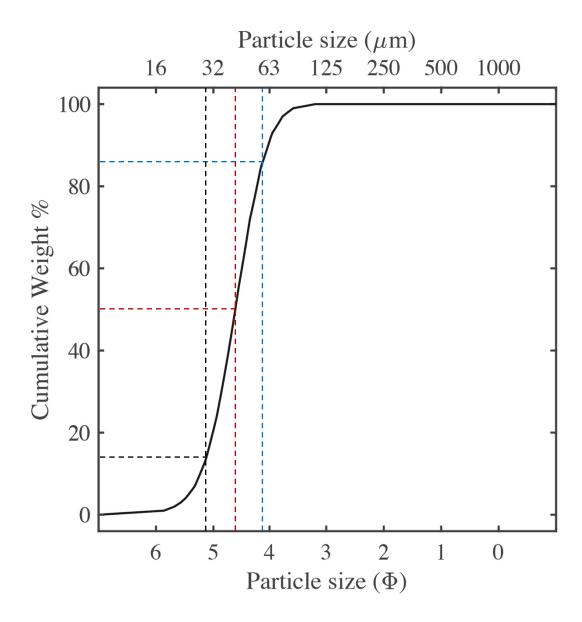
**Supplementary Figure 1.** Cumulative grain size distribution of the glass beads used in the experiments ( $D_{50} = 41.5 \mu m$ ,  $\sigma = 14 \mu m$ ). The grain size distribution was obtained by laser diffraction using a BetterSizer S3 Plus. The dotted black, red and blue lines respectively indicate the 14<sup>th</sup>, 50<sup>th</sup> and 86<sup>th</sup> percentiles.
