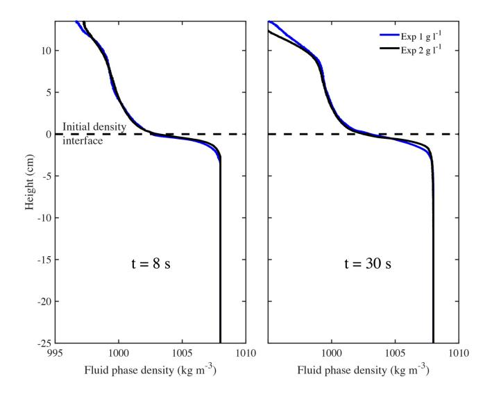
**Supplementary Figure 2.** Comparison of the fluid density profiles for experiments A11 and A12 (with particle concentrations of 1 and 2 g l<sup>-1</sup>, respectively). Results are very similar and reproducible.
