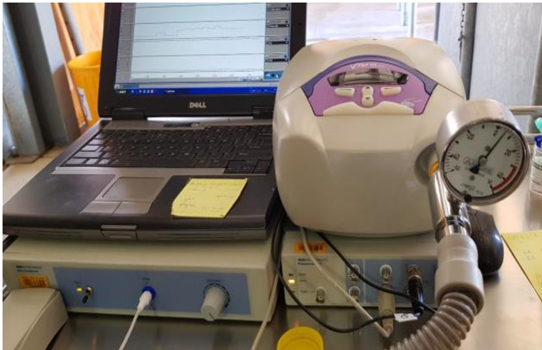
Supplementary Figure S1: BiPAP ventilator, spirometer and gas analyser (top), mask with vented non-rebreathing elbow valve (A) and spirometry flow head (B). Oxygen was added to the circuit at C.
