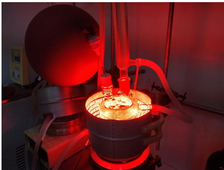
Figure S1. Picture of one of the two thermoregulated batch reactors used this study
