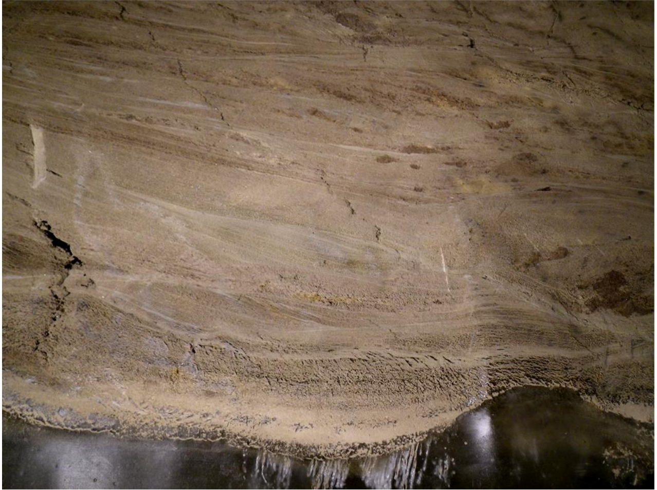
Figure S19. Stratified and cross-stratified silt and silty sand with numerous inclusions of the organic matter reworked by fluvial processes; note thermokarst-cave ice at the bottom (see Figure S18 ); the boundary between stratified sediments and massive ice may be interpreted as an erosion unconformity. Right wall of the main adit of the new tunnel (T2), distance 38.6-39.1 m, elevation 229.5-229.9 m (for location, see Figures 6 and 7 ).
