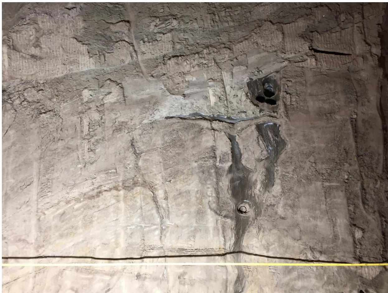
Figure S43. Pleistocene/Holocene boundary (thaw unconformity marked by truncated ice wedges and lenses). Right wall of Crosscut #1 of the new tunnel (C1), distance 41.0-44.0 m, elevation 228.8-231.0 m (for location and interpretation, see Figure 10 ).
