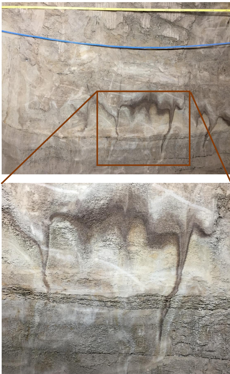
Figure S33. Organic-rich silt with micro-cryostructures and ice belts typical of undisturbed Yedoma. Note turbated organic-rich layers in Yedoma silt. Left wall of Crosscut #1 of the new tunnel (C1), distance 18.4-19.8 m, elevation 228.1-229.0 m (for location, see Figure 10 ).
