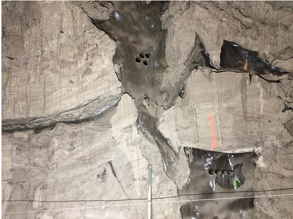
Figure S21. Ice wedge truncated by thermal erosion; bodies of thermokarst-cave ice were crossed by the ice wedge of younger generation. Left wall of the main adit of the new tunnel (T2), distance 66.0-70.8 m, elevation 228.7-231.6 m (for location and interpretation, see Figure 6 ).
