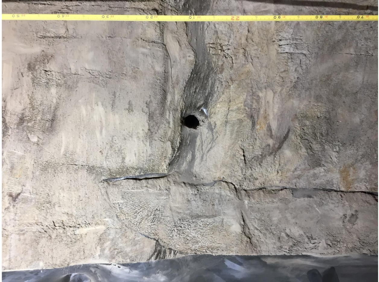
Figure S44. Underground erosional channel filled with silt with reticulate-chaotic cryostructure; underlain by large thermokarst-cave ice body. Right wall of Crosscut #1 of the new tunnel (C1), distance 41.7-42.5 m, elevation 228.3-229.0 m (for location and interpretation, see Figure 10 ).
