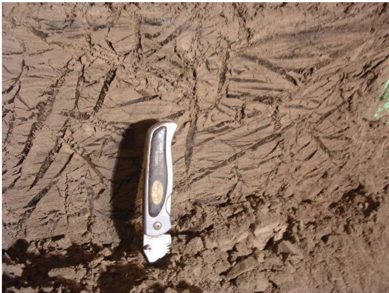
Figure S8. Photograph of the reticulate-chaotic cryostructure (the handle of the knife is about 6 cm long) (Fortier et al., 2008).
