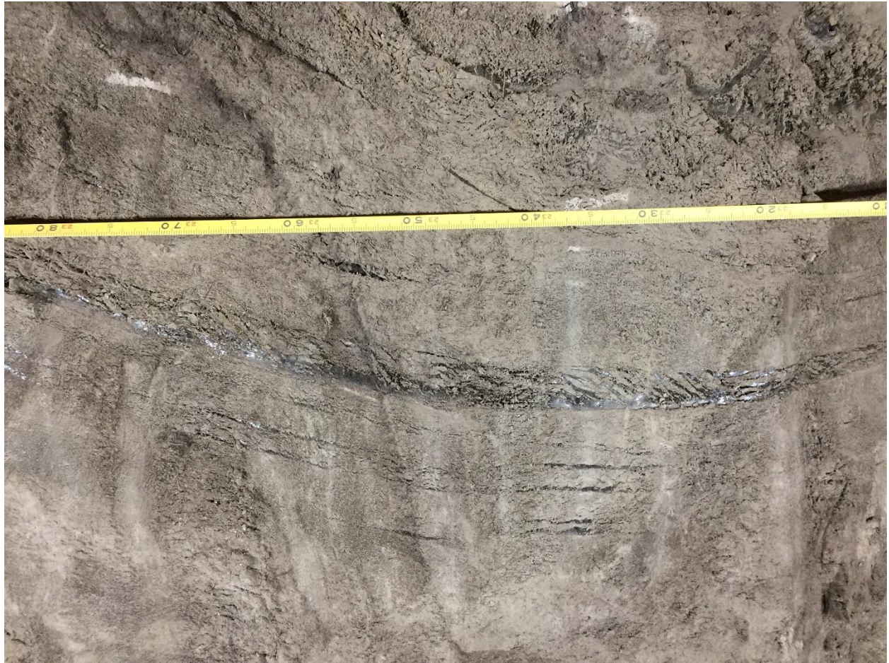
Figure S37. Syngenetically frozen Yedoma silt with ice belts and micro-cryostructures. Right wall of Crosscut #1 of the new tunnel (C1), distance 23.1-23.8 m, elevation 228.7-229.2 m (for location, see Figure 10 ).
