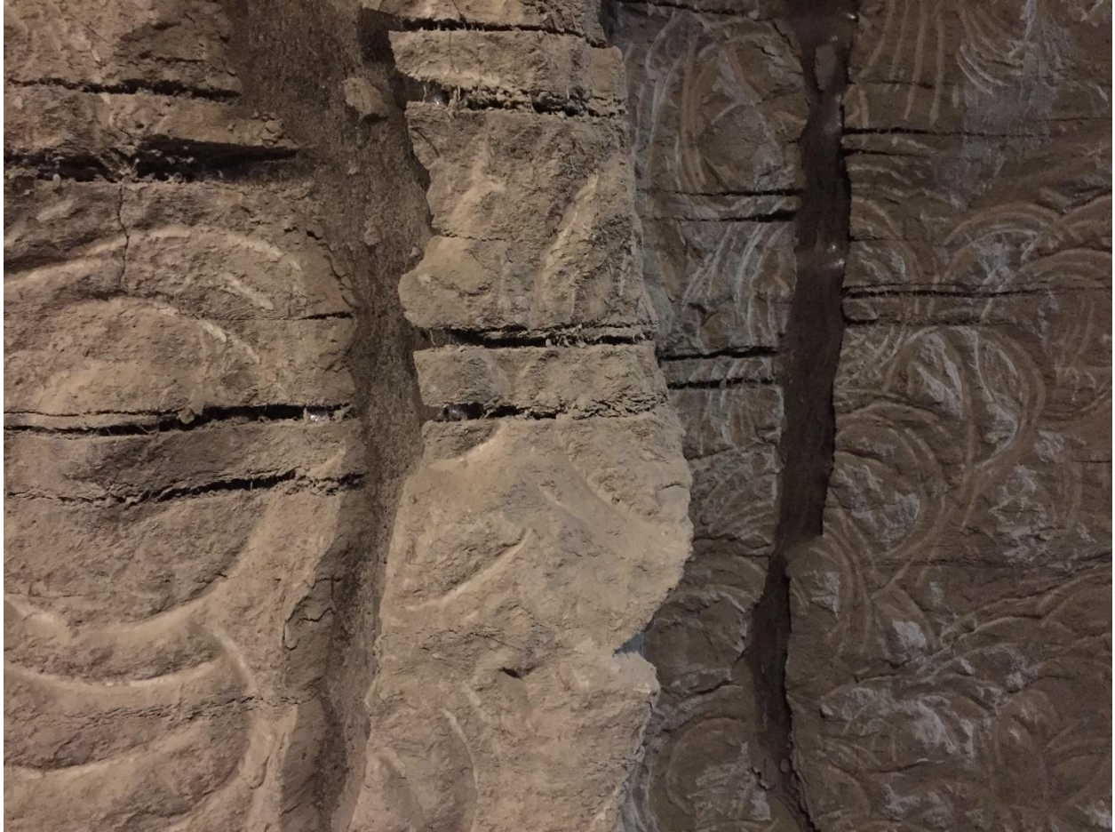
Figure S27. Displacements of ice belts along a small ice wedge, right wall of the main adit of the new tunnel (T2), distance approximately 92.6-93.8 m, elevation 230.2-230.7 m (for location, see Figure 6 ).
