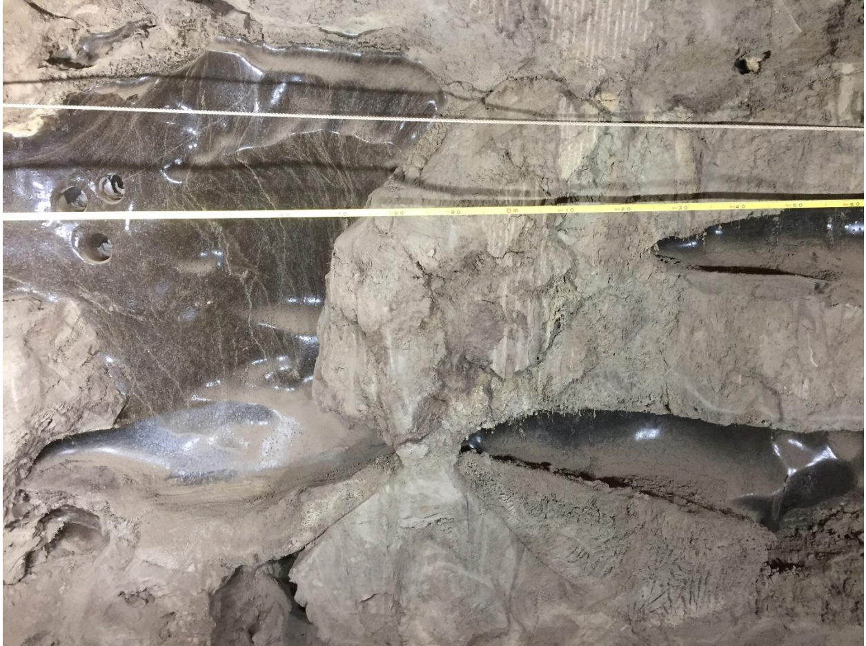
Figure S38. Underground erosional channels filled with thermokarst-cave ice underlain by silt with reticulate-chaotic cryostructure. The channels started developing along ice wedges but eventually expanded and affected enclosing sediments. Left wall of Crosscut #1 of the new tunnel (C1), distance 27.0-28.6 m, elevation 228.2-229.4 m (for location and interpretation, see Figure 10 ).
