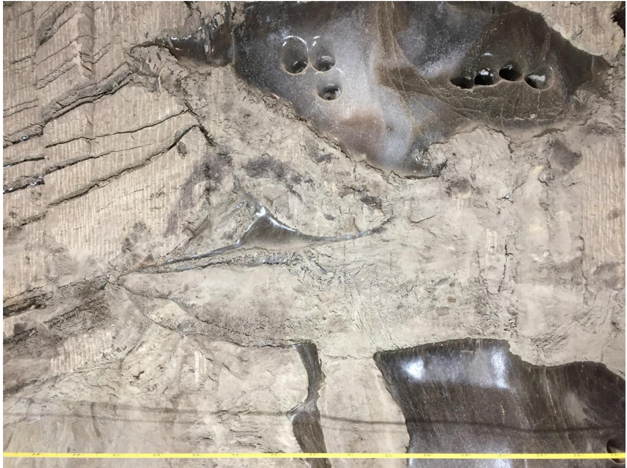
Figure S34. Ice wedge truncated by thermal erosion and underground channels filled with thermokarst-cave ice and silt with inclusions of reworked organic matter. Right wall of Crosscut #1 of the new tunnel (C1), distance 16.4-18.0 m, elevation 229.0-230.2 m (for location and interpretation, see Figure 10 ).
