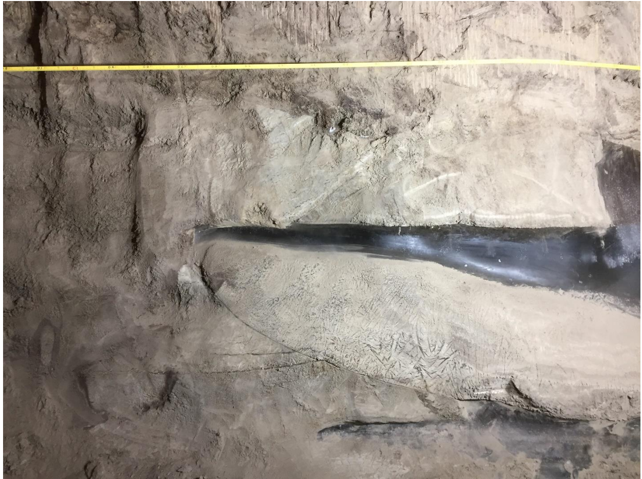
Figure S41. Thermokarst-cave ice underlain by silt with reticulate-chaotic cryostructure. Right wall of Crosscut #1 of the new tunnel (C1), distance 31.2-33.2 m, elevation 227.7-229.2 m (for location, see Figure 10 ).
