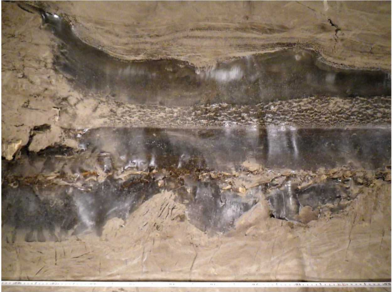
Figure S18. Thermokarst-cave ice (see Figure S16 ); horizontal stratification and suspended wood fragments indicate several stages of water accumulation and thermokarst-cave ice aggradation in the underground cavity. Right wall of the main adit of the new tunnel (T2), distance 38.9-39.9 m, elevation 229.0-229.9 m (for location, see Figures 6 and 7 ).
