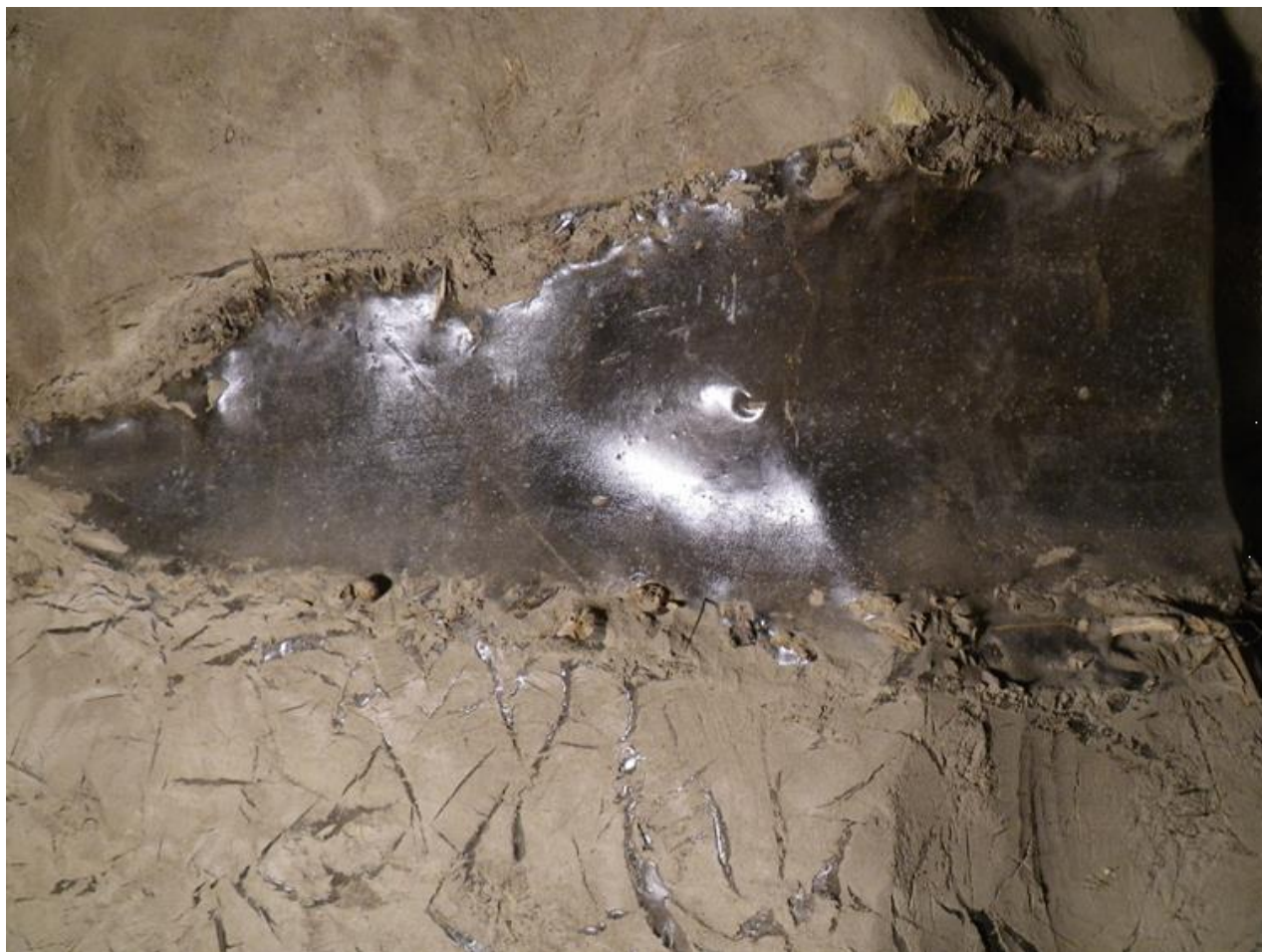
Figure S17. Thermokarst-cave ice (see Figure S16 ) underlain by silt with reticulate-chaotic cryostructure; note the presence of woody debris in the silt at the bottom of the thermokarst-cave ice body. Right wall of the main adit of the new tunnel (T2), distance 41.8-42.5 m, elevation 229.2-229.6 m (for location, see Figures 6 and 7 ).
