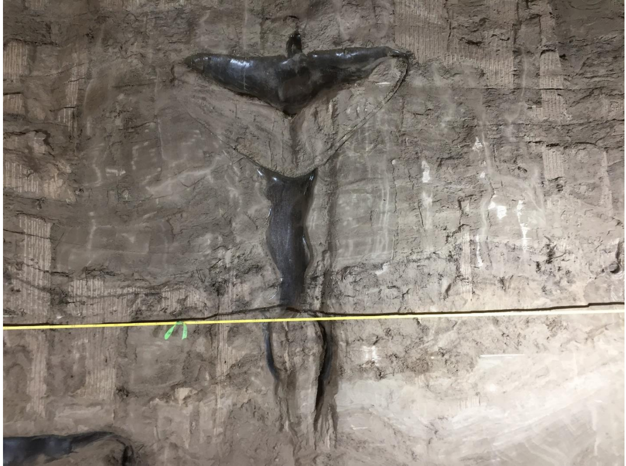
Figure S40. Ice wedge truncated by thermal erosion; underground channel filled with thermokarst-cave ice underlain by silt with reticulate-chaotic cryostructure. Right wall of Crosscut #1 of the new tunnel (C1), distance 29.0-30.8 m, elevation 228.3-230.7 m (for location, see Figure 10 ).
