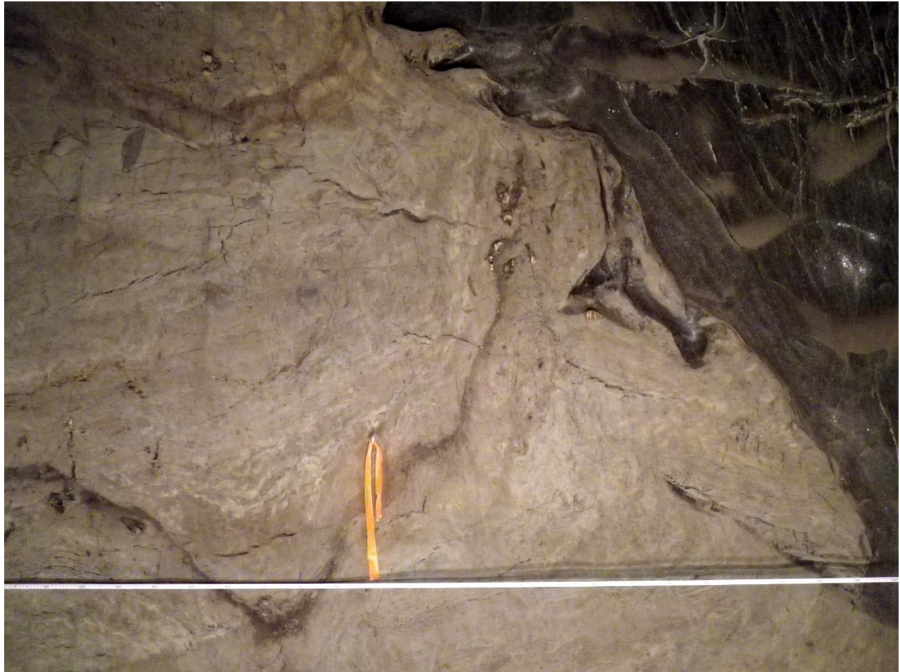
Figure S15. Large Late Pleistocene ice wedge and deformed peat layers. Left wall of the main adit of the new tunnel (T2), distance 31.0-33.5 m, elevation 228.7-230.6 m (for location, see Figure 6 ).
