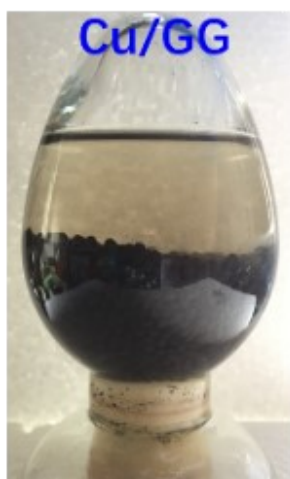
Figure s1 the stability testing of spherical hydrogel after standing for 1 year, the concentration of metal ions is 100 mM.
