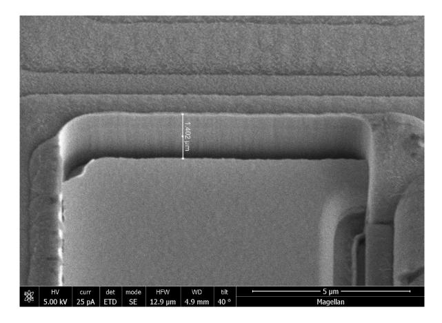
SEM image of a recessed electrode on the CMOS chip surface with indicated projected feature height h.
