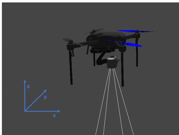
**Supplementary Fig. S1.** An IRIS UAV model in the Gazebo simulation using ardupilot software in the loop (SITL) as a flight controller.
