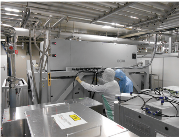
Figure 15: New CO 2 laser pre-AMP for the 20-kW CO 2 laser system.
