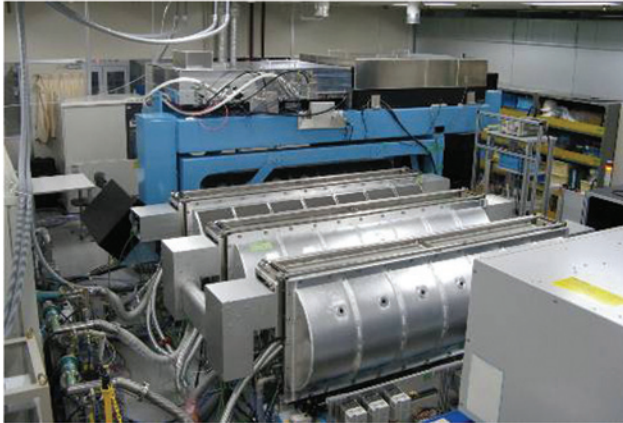
Figure 7: Driver CO 2 laser system test at Mitsubishi Electric.
