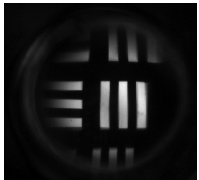
Figure 8: Imaging test of the endoscope.
