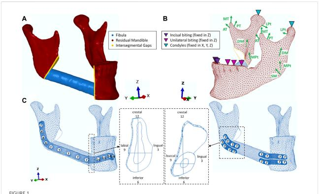
(A) geometry without fixation; (B) loading and boundary conditions including muscles superficial- (SM) and deep (DM) masseter, medial- (MPt) and lateral (LPt) pterygoid, anterior- (AT), medial- (MT) and posterior (PT) temporalis; (C) reconstruction plate and miniplate with screws and screw lengths (in mm), intersegmental gaps with anatomical and given clock directions.
