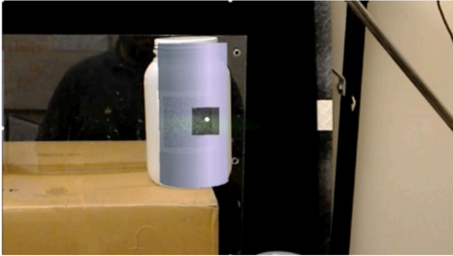
FIGURE 20 | The holographic button associated with the cursor is actuated using the cursor and a “select” voice command.
