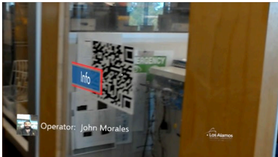
FIGURE 12 | The doors of the mock facility have been instrumented with QR codes. The augmented reality headset can recognize the QR codes. A holographic interface can provide information to the operator regarding the contents of the room if they air-tap the info.
