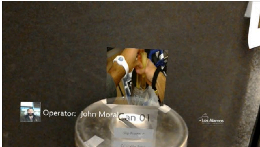
FIGURE 9 | The holographic display can be used to display video of the process of loading the canister which is important for documentation requirements in certain nuclear facilities.
