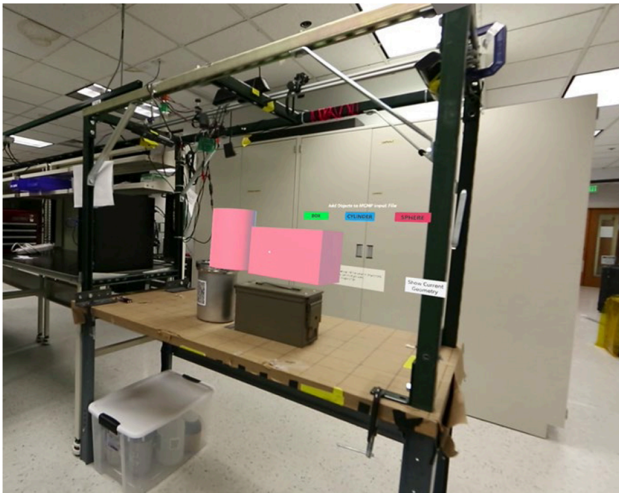
FIGURE 30 | 3rd-person view of a human operator using an augmented reality headset to determine the geometry for MCNP input files in-situ .
