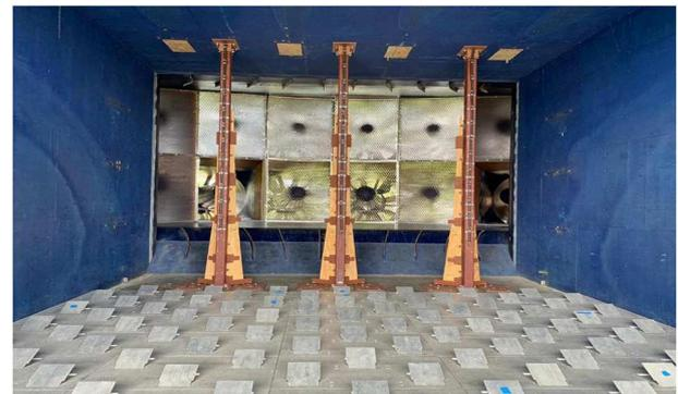
**FIGURE 2** | Spires and floor roughness elements in the WOW flow management section.
