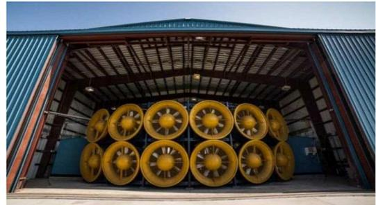
**FIGURE 1** | Intake of 12-fan Wall of Wind system.
