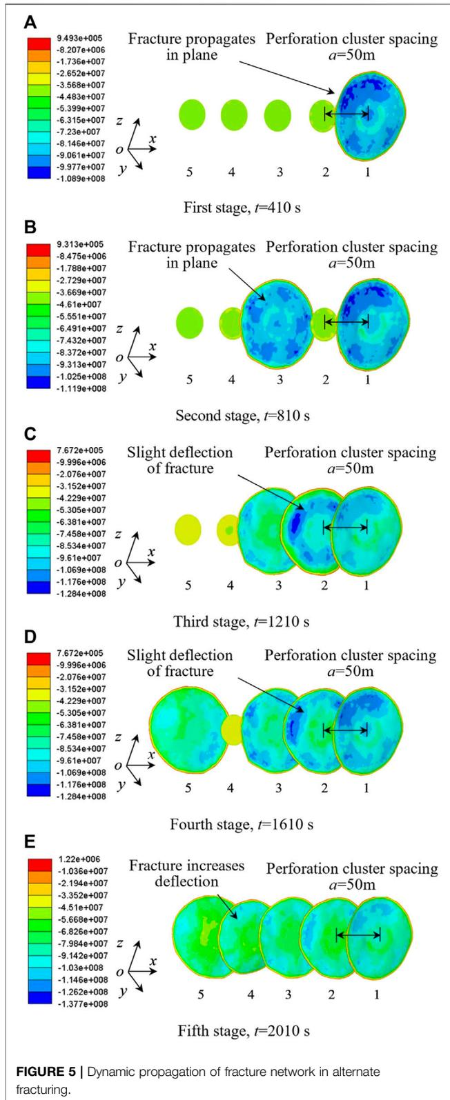
**FIGURE 5** | Dynamic propagation of fracture network in alternate fracturing.
