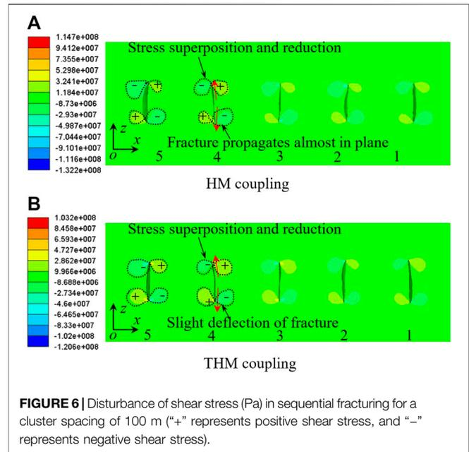
**FIGURE 6** | Disturbance of shear stress (Pa) in sequential fracturing for a cluster spacing of 100 m (“+” represents positive shear stress, and “-” represents negative shear stress).
