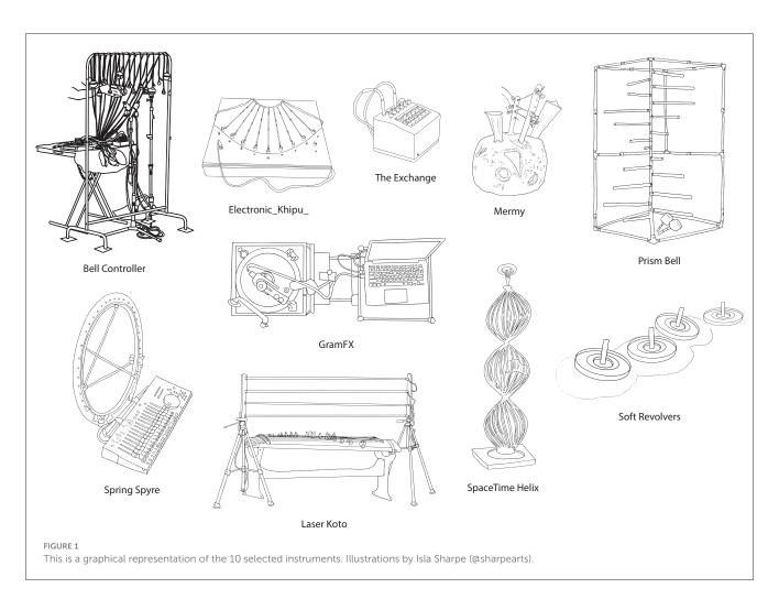
**Soft Revolvers**,<sup>7</sup> created by Myriam Bleau in 2014, are spinning tops with embedded sensors that trigger sound samples.
