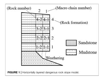
10.31 m (the penetration rate is 62.5%) that is caused by weathering (**Figure 1**). According to the specification of Chen et al. (2009a), the studied slope of dangerous rock is ascribed to the falling damage group. The stability calculation method of different weathering degree of dangerous rock with seismic transverse and longitudinal waves is obtained to judge the effective seismic wave corresponding to different models.
