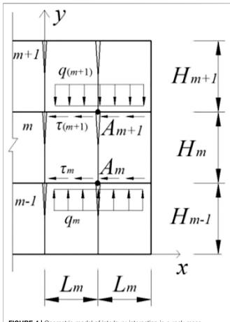
FIGURE 4 | Geometric model of interlayer interaction in a rock mass.
