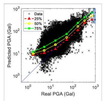
FIGURE 9 Comparison between the predicted PGA and actual PGA of the entire TSMIP data set using the proposed LSTM approach. The distribution of the earthquakes with real PGA larger than 800 Gal is marked with the blue box.
