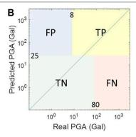
FIGURE 5 | The confusion matrix when the threshold is designated as 25 Gal (A) without tolerance, and (B) with tolerance. FP is false positive; FN is false negative; TP is true positive; and TN is true negative.
