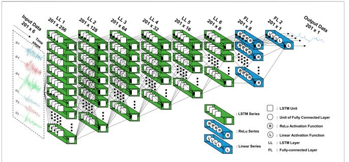
FIGURE 4 | Proposed architecture of the LSTM model. LL 1 is the 1st LSTM Layer; LL 2 is the 2nd LSTM Layer and so on; FL 1 is the 1st Fully-connected Layer; FL 2 is the 2nd Fully-connected Layer.
