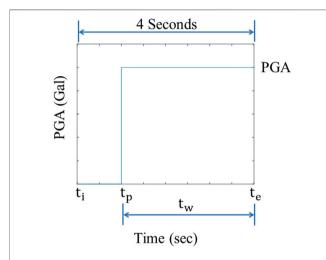
**FIGURE 2** | The schematic diagram of the target output of the LSTM model.  $t_p$  is the P-wave arrival time;  $t_i$  and  $t_e$  are start time and end time, respectively; and  $t_w$  is the length of the time-window between  $t_p$  and  $t_e$ .
