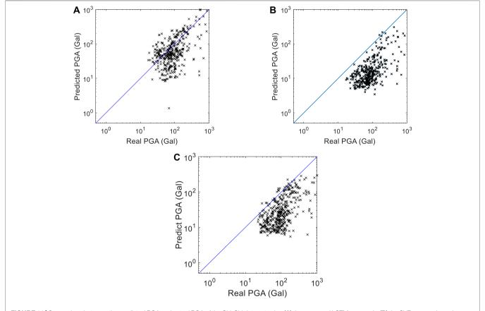
FIGURE 11 | Comparison between the predicted PGA and actual PGA of the Chi-Chi data set using (A) the proposed LSTM approach, (B) the SVR approach, and (C) the CNN approach.
