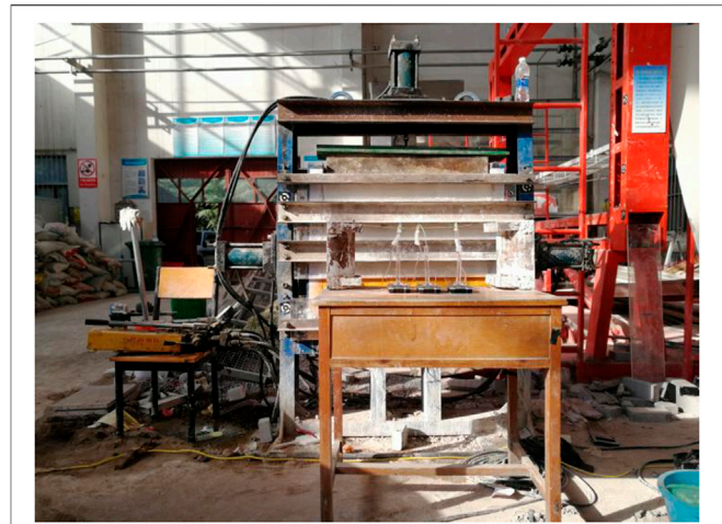
FIGURE 2 | Borehole deformation similarity simulation test system.
