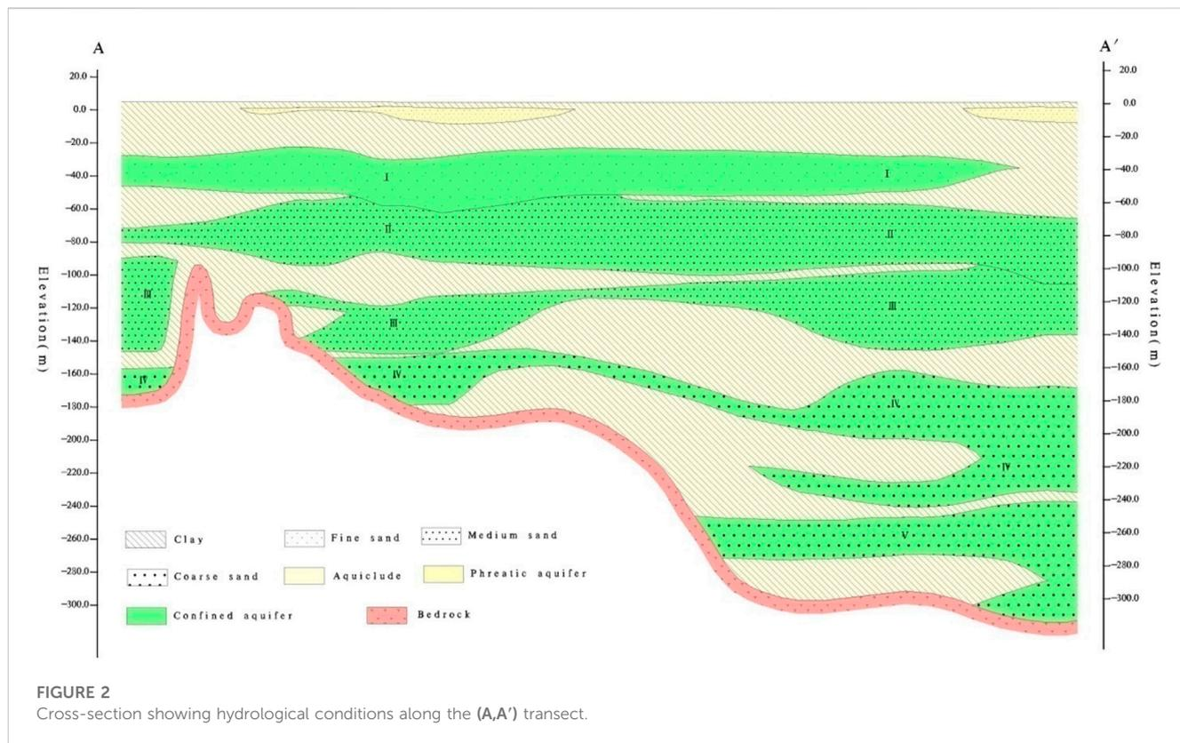
FIGURE 2 Cross-section showing hydrological conditions along the (A,A') transect.
