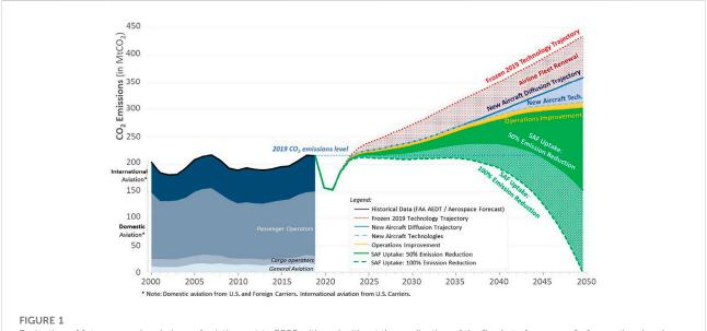
Projection of future annual emissions of aviation out to 2050 with and without the application of the "basket of measures" of operational and technological advancements and SAF deployment. Without SAF, the aviation sector will not meet the net-zero emissions goals they have set. Source (United States, 2021) used with permission.
