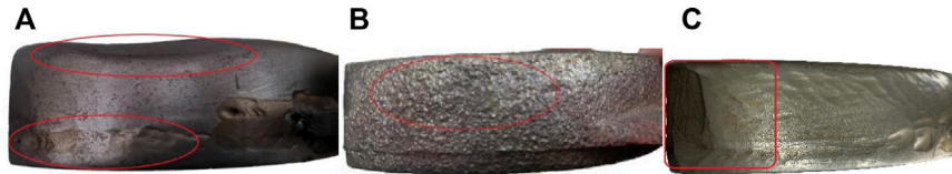
FIGURE 15 | Pressure surface wear under different materials. (A) 16 Mn, (B) HT200, and (C) Q235.
