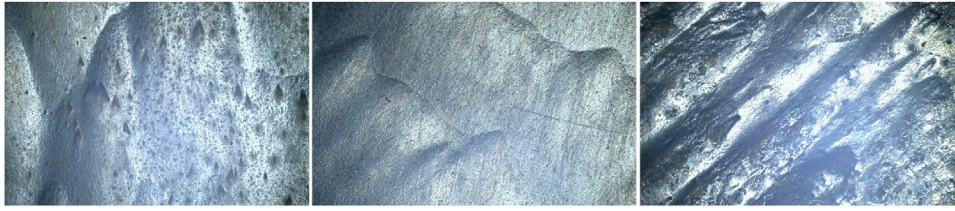
FIGURE 17 | Surface micrographs of the trailing edge of the blade wear different material.
