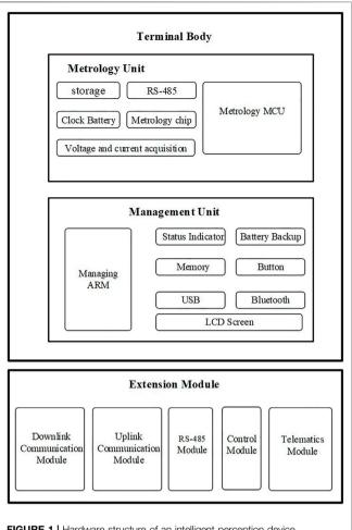
FIGURE 1 | Hardware structure of an intelligent perception device.
