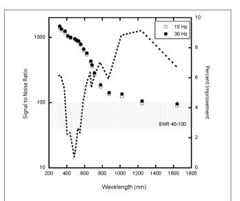
**FIGURE 7** Effective signal-to-noise ratio (SNR) calculated at LSA for C-AERO data over Monterey Bay, CA collected 26 October 2018 (C-HARRIER) with C-AERO at 15 and 30 Hz. The stippled region identifies an optimal SNR of 40–100, while the dashed line provides the percent difference in SNR for 15 versus 30 Hz otherwise processed using the same methods. The percent improvement (as percent increase in SNR when collecting at 15 versus 30 Hz) is shown as the dashed line.
