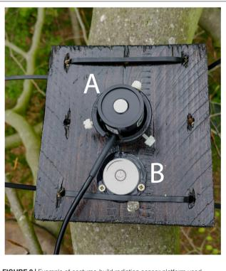
FIGURE 2 | Example of costume-build radiation sensor platform used, showing the pyranometer (A) and a spirit level (B).
