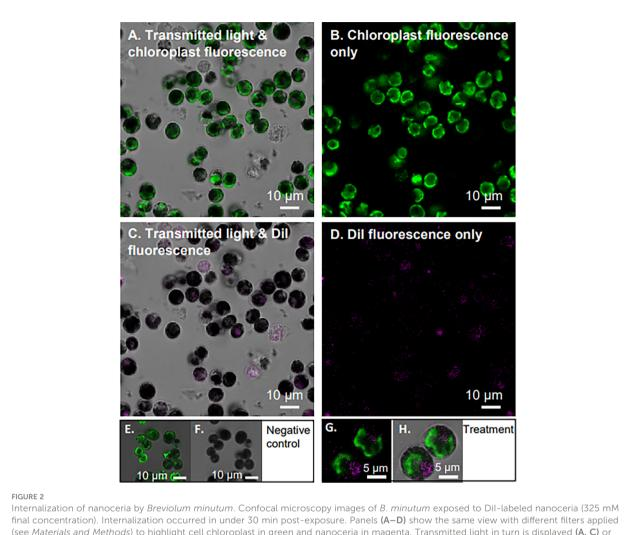
final concentration). Internalization occurred in under 30 min post-exposure. Panels (A–D) show the same view with different filters applie (see *Materials and Methods*) to highlight cell chloroplast in green and nanoceria in magenta. Transmitted light in turn is displayed (A, C) or not (B, D) for contrast. Images of negative control are also displayed (E, F). Enlarged view of two *B. minutum* cells with internalized Dillabeled nanoceria (G, H). Scale bars: (A–F) 10 µm; (G, H) 5 µm.
