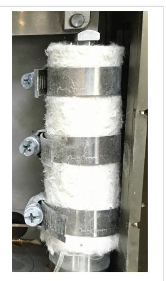
FIGURE 7 | Photograph of the piezostack actuator with the heat insulation.
