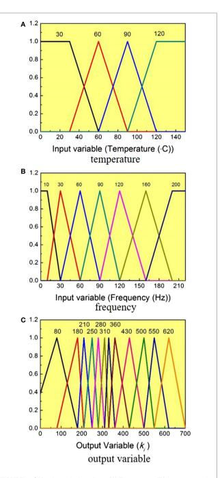
FIGURE 11 | Membership functions. (A) Temperature, (B) frequency, and (C) output variable.
