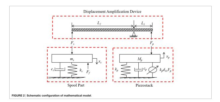
$$m_{p}\ddot{x}_{p} + c_{p}\dot{x}_{p} + k_{p}x_{p} = k_{p}d_{33}V_{p} - F_{p}$$
