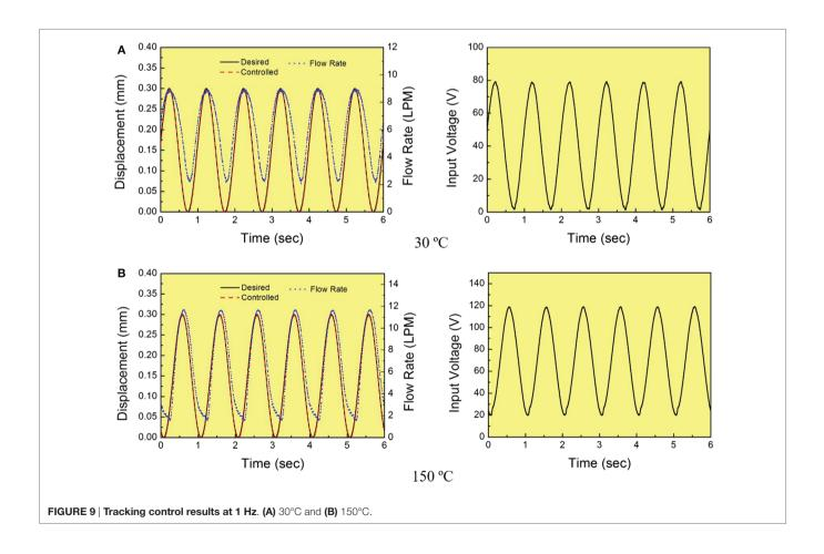
is not enough to operate up to 200 Hz without delay. Therefore, the stiffness will be designed much higher for the valve system in the next study. However, the time delay is not directly related to the operating temperature. The used simple PID controller has good performance with fixed conditions such as 150°C and 200 Hz,
