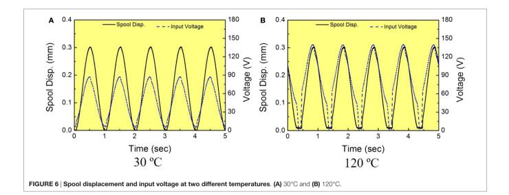
has slow response time. Therefore, in this work, control target is selected as the displacement of the spool instead of the flow rate to accommodate high excitation frequency. It is remarked that the response time of the displacement sensor is sufficiently fast to acquire the signal occurred at the excitation frequency of 200 Hz.
