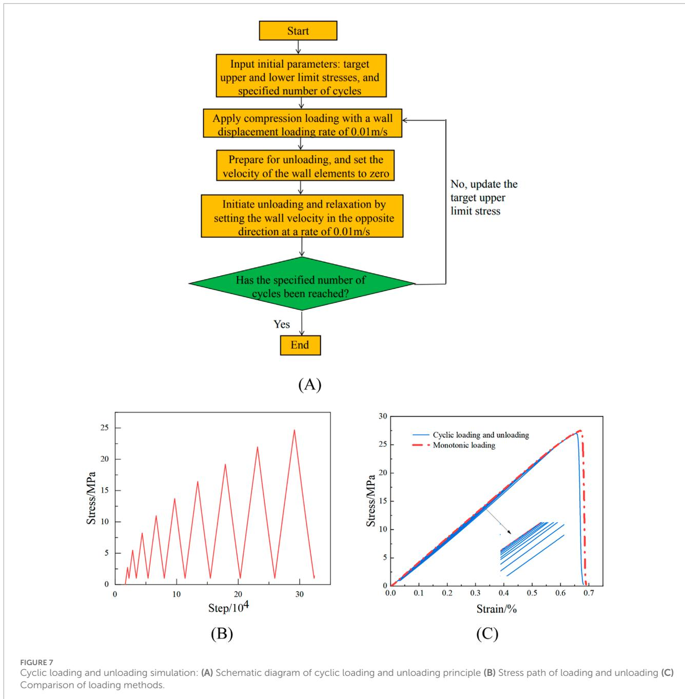
**FIGURE 7** Cyclic loading and unloading simulation: **(A)** Schematic diagram of cyclic loading and unloading principle **(B)** Stress path of loading and unloading **(C)** Comparison of loading methods.
