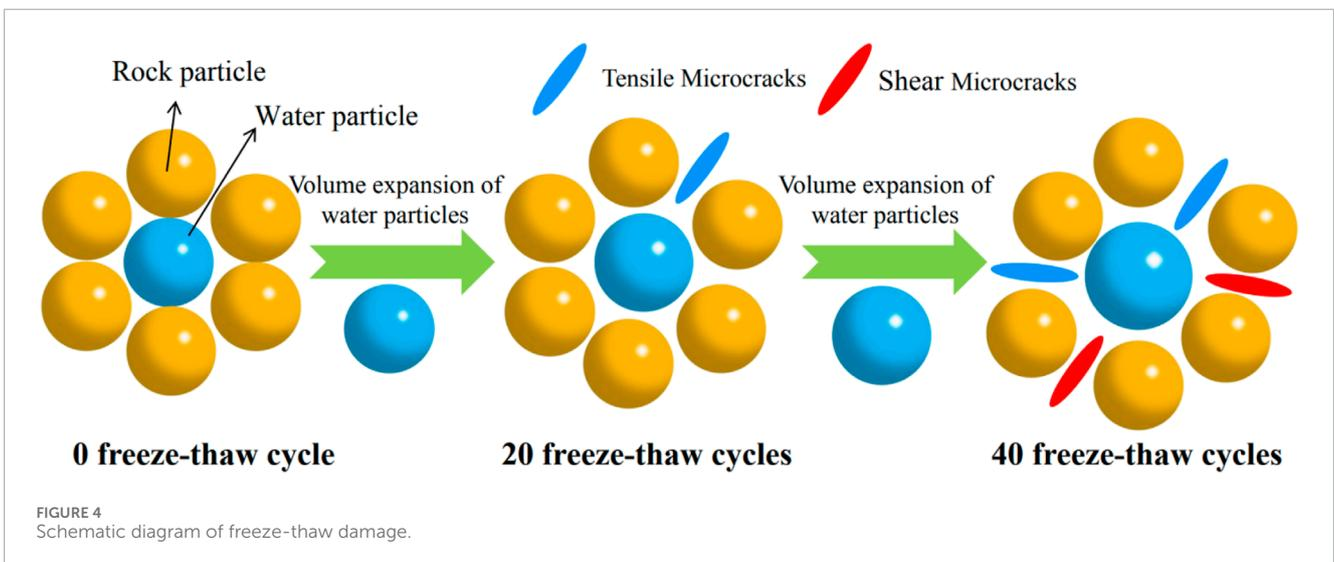
cycle are almost similar. An escalation in freeze-thaw cycles leads to an increase in microcracks inside the rock, less deformation resistance, and a decline in the elastic modulus. The aforementioned calibrated microscopic parameters are rational and practicable.
