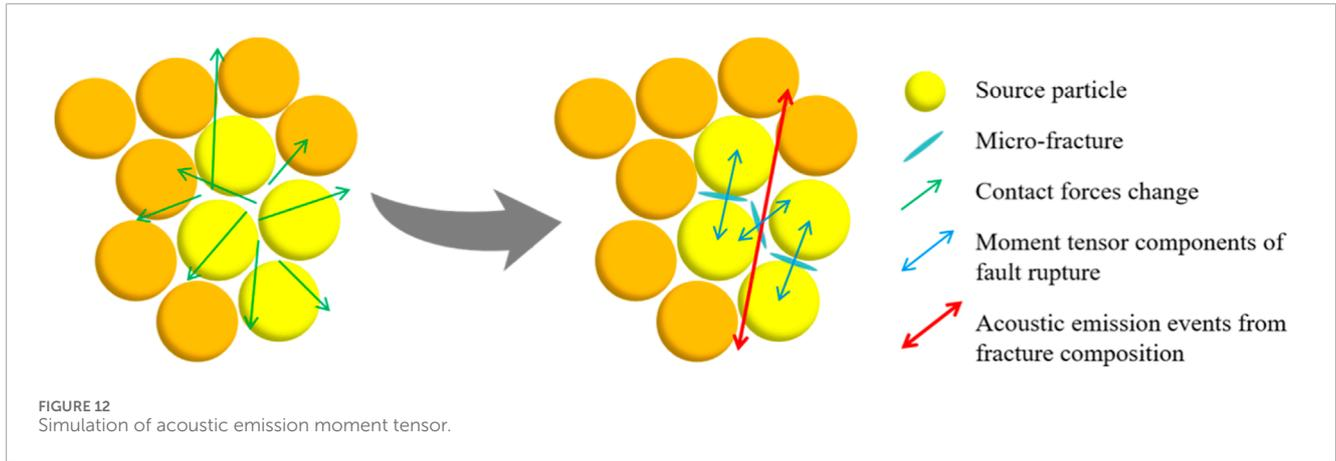
the emergence of numerous micro-fractures. Under load, micro-cracks in a certain area are more likely to converge and form macroscopic cracks within a short period of time, releasing high-magnitude signals and resulting in large-scale cracks. The fatigue damage caused by cyclic loading facilitates the propagation and extension of micro-fractures as well as the frictional slip between crack surfaces, making the sample more prone to large-scale failure.
