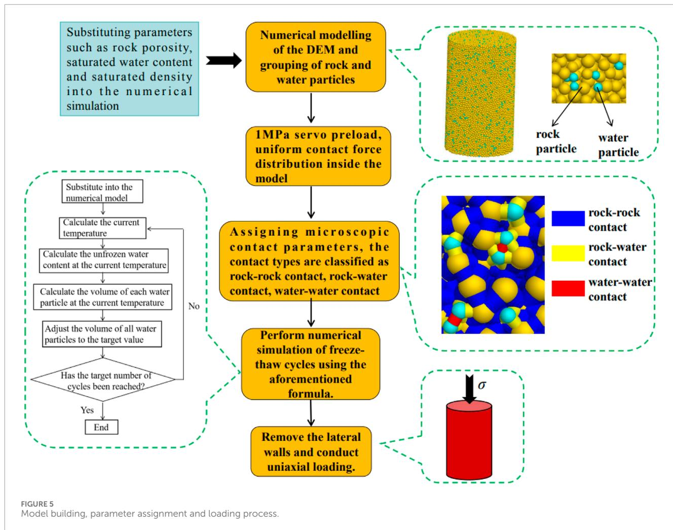
FIGURE 5 Model building, parameter assignment and loading process.
