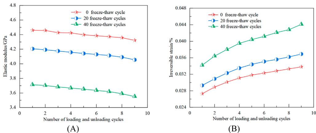
**FIGURE 8** Changes of elastic modulus and irreversible strain under cyclic loading and unloading condition: **(A)** Change in elastic modulus **(B)** Irreversible strain change.
