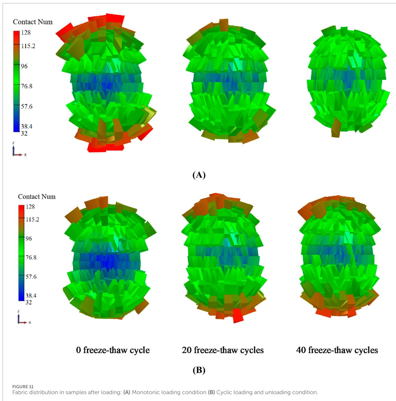
FIGURE 11 Fabric distribution in samples after loading: (A) Monotonic loading condition (B) Cyclic loading and unloading condition.
