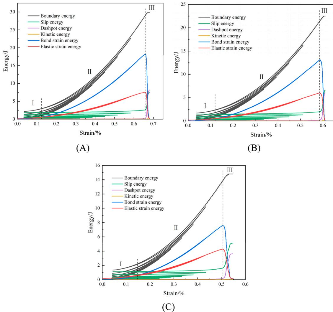
FIGURE 15 Energy evolution law at the mesoscale of sandstone under different freeze-thaw cycles: (A) 0 freeze-thaw cycle (B) 20 freeze-thaw cycles (C) 40 freeze-thaw cycles.
