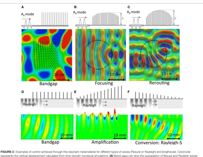
leaving desired regions free of vibrations. (**B**,**C**) Elastic energy can be guided or focused with gradient index lenses. (**D**) Rayleigh wave band-gap created by the constant height resonators. (**E**) Waves can be spatially segregated depending on the frequency and strongly amplified. (**F**) Rayleigh waves can be converted to S-waves and redirected in the bulk. The aspect ratio of the rods and the height gradient are not in scale to better present the concept.
