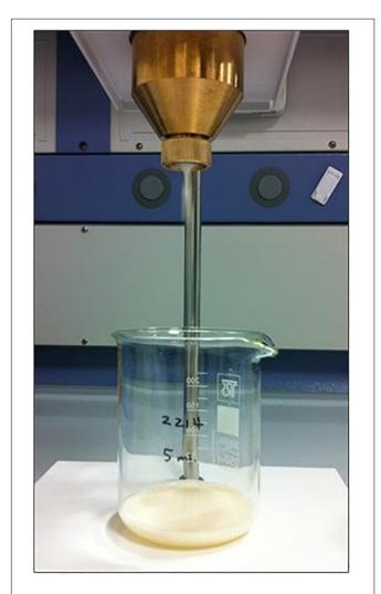
**FIGURE 2** Ford cup used to measure the viscosity of fermented milk by weighing the milk flowing through an orifice of 3 mm diameter.
