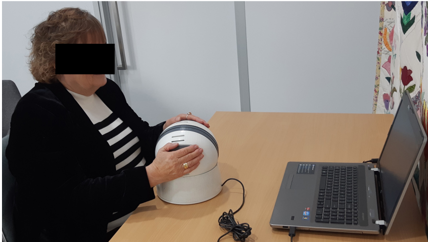
FIGURE 1 | The Orby Controller, which consists of several features specifically adapted for motor dysfunction, including: (1) a spherical shape to allow for ergonomic bimanual control, (2) gray grip pads (partially obscured during use) and optional hand straps to support hand placement, (3) an adjustable sensitivity threshold, to prevent random movements from being interpreted as purposeful, (4) vibration to provide haptic feedback to the player, and (5) a large red selection button on the front of the controller to reduce the fine motor requirement (not shown).
