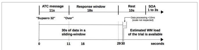
FIGURE 6 | Trial timeline and computing latencies. Upper timeline shows ATC span task trial events duration (see Figure 3). Bottom timeline illustrates duration constraints to get pilot's estimated WM load: classifier's response is available in the worst case less than 10 ms after pilot's response window.
