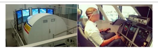
FIGURE 2 | (Left) ISAE-Supaero flight simulator; the closed cabin is visible from rear, and eight screens are used to visualize external environment. (Right) The pilot subject with the fNIRS headband.
