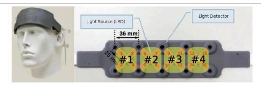
FIGURE 1 | fNIR Device® Model 1200S headband and associated optode numbering. Only the four closest detectors to an emitter constituted optodes. Optodes are represented in red with their associated number. Four regions of interest (ROI) were defined for statistical analyses purposes (#1, #2, #3, #4).
