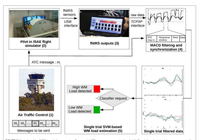
FIGURE 5 | Illustration of the fNIRS based inference system. Pre-recorded ATC messages were sent to the pilot (1). The pilot's prefrontal activity was measured with a fNIRS device (2). Output measures (3) were MACD-filtered and synchronized with the temporal design of the trial (4). When all of the required data were available for the trial, a request was sent to the pilot's classifier to assess the WM load of the trial (5).
