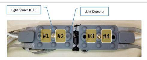
FIGURE 7 | Miniaturized and wireless fNIR Device<sup>®</sup> Model 1200W headband and associated regions of interest (optodes). Optodes are represented in yellow with their associated number.
