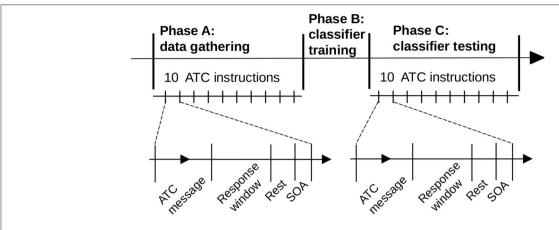
**FIGURE 4** | The experiment was split into three successive phases. Data gathering (phase A) and classifier testing (phase C) consisted of 10 ATC instructions each. The pilot's classifier was trained between these two phases (phase B). The time scale of the figure is illustrative.
