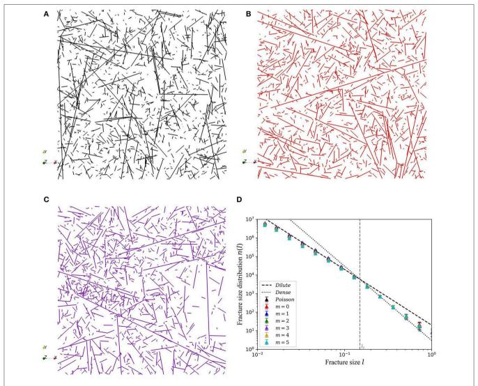
**FIGURE 2** | 2D slices of three-dimensional **(A)** Poisson, **(B)** stress-independent UFM ( $\mathbf{m} = \mathbf{0}$ ), and **(C)** stress-driven UFM ( $\mathbf{m} = \mathbf{3}$ ) models, and **(D)** associated size distributions ( $\mathbf{m} \in [0, \mathbf{5}]$ ).
