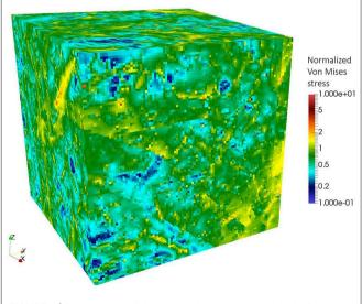
**FIGURE 1 |** Stress-intensity field generated on a regular grid of size  $\mathbf{L}=\mathbf{1}$  and resolution  $\mathbf{r}=\mathbf{0.01}.$
