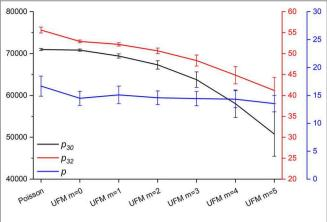
**FIGURE 3** | Fracture density statistics of generated networks in cubic systems of volume V = 1.
