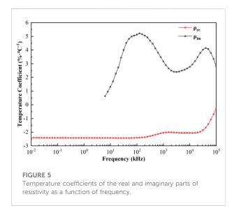
between the imaginary part and temperature at each frequency, with a coefficient of determination $\geq 0.969$ . We borrowed the method of (Jaspard and Nadi 2002) and used Eq. 4 to calculate the temperature coefficients of the real and imaginary parts of the blood resistivity at each frequency.
