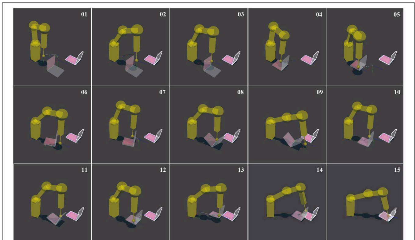
FIGURE 6 | Simulation of a Katana robot arm equipped with a spherical finger that plans a sequence of pushes to move an L-shaped object, called polyflap (Sloman, 2006) to a goal state. The plan is created by using a physics engine (PhysX) to predict the outcome of a push operation. Image 01 shows the initial pose. The wire-framed L-shaped polyflap is a “phantom” to indicate the desired goal state. The goal pose is translated from the initial pose by 28 cm and rotated by 90°. Image 02 shows the collision-free trajectory to bring the end effector to the start pose of the first push. Images 01–04 show the first push which makes the polyflap tip over. Images 05–09 show a series of pushes which culminate in the polyflap resting in an unstable equilibrium pose along its folded edge. Images 12 and 13 show a sideways push. Images 14 and 15 show the final frontal push which aligns the polyflap with the target configuration. Courtesy of Zito et al. (2012).
