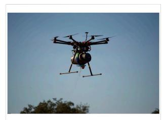
**FIGURE 2**DJI S1000 + octocopter with the vermiculite dispenser "Bugbot" attached.
