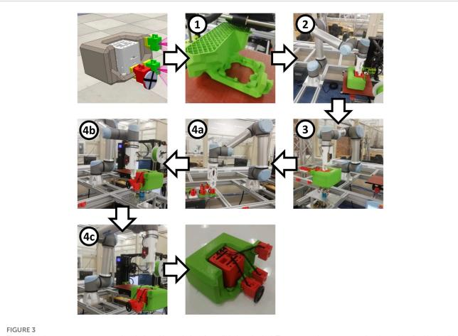
The production process to create a robot designed by evolution, from digital to physical. The step numbers correspond to those described in detail in the main text. Firstly the skeleton must be 3D printed before the head (containing the controller and battery) is inserted. Then wheels and sensors can be attached and connected to the head via retracting cables. The complete process of producing a physical robot from its digital specification is done autonomously.
