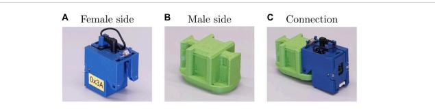
This figure shows the mechanical connector used in the ARE platform. The female side (A) uses two sprung arms to engage with the indentations on the male side (B) to form the final connection (C).
