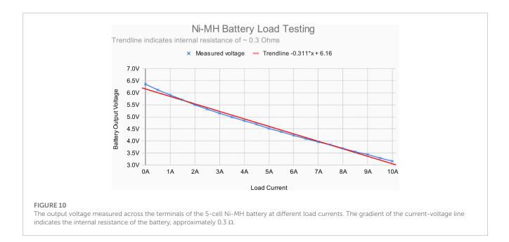
around 3.5 A. For context, this would accommodate only two joint servos at their maximum 1.25 A current limit, if allowing 1 A for the microcontroller and internal components. Robots with sensors and current-limited wheel organs could be built, but current limiting would be essential, and most limbs would be unachievable.
