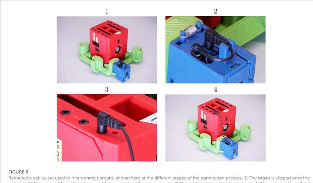
Retractable cables are used to interconnect organs, shown here at the different stages of the connection process: 1) The organ is clipped onto the skeleton. 2) The retractable cable is drawn out from a cavity in the organ casing. 3) The cable is connected to the head. 4) The coiled cable self-adjusts its length to the distance between the head and the organ.
