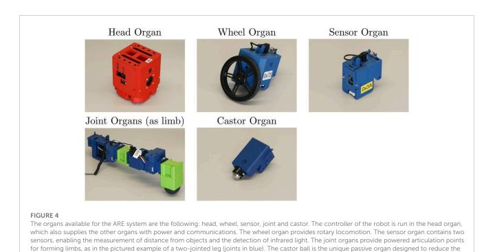
The leg organ is a two-jointed construct of these combined with a rubber-tipped foot. There is also an additional passive organ with no electronics, the castor organ, which is a simple ball castor enabling evolution to generate free-rolling points on a robot. The organ types and their functionality are summarised in Figure 4.
