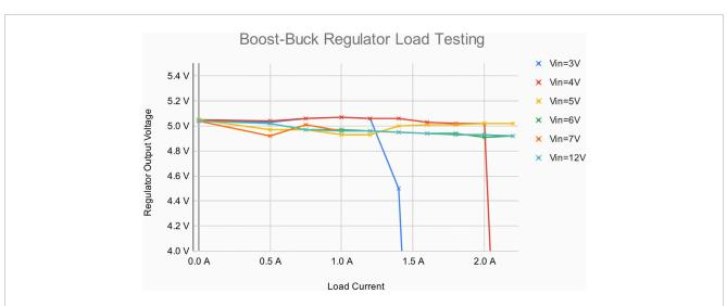
The output voltage measured at the output of the boost-buck regulator circuit at different load currents and input voltages, showing that it can easily step down from higher voltages, but the extra switch current required in boost mode limits how low the input voltage can go. Sudden drops indicate thermal cutout of the regulator, showing the limits of its output capability.
