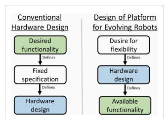
An illustration of how the hardware design paradigm changes for an evolvable robot platform. Rather than the design being defined by fixed constraints derived from the desired functionality for the robot, the hardware design comes first, and defines the constraints on the functionality available to the evolved robots.
